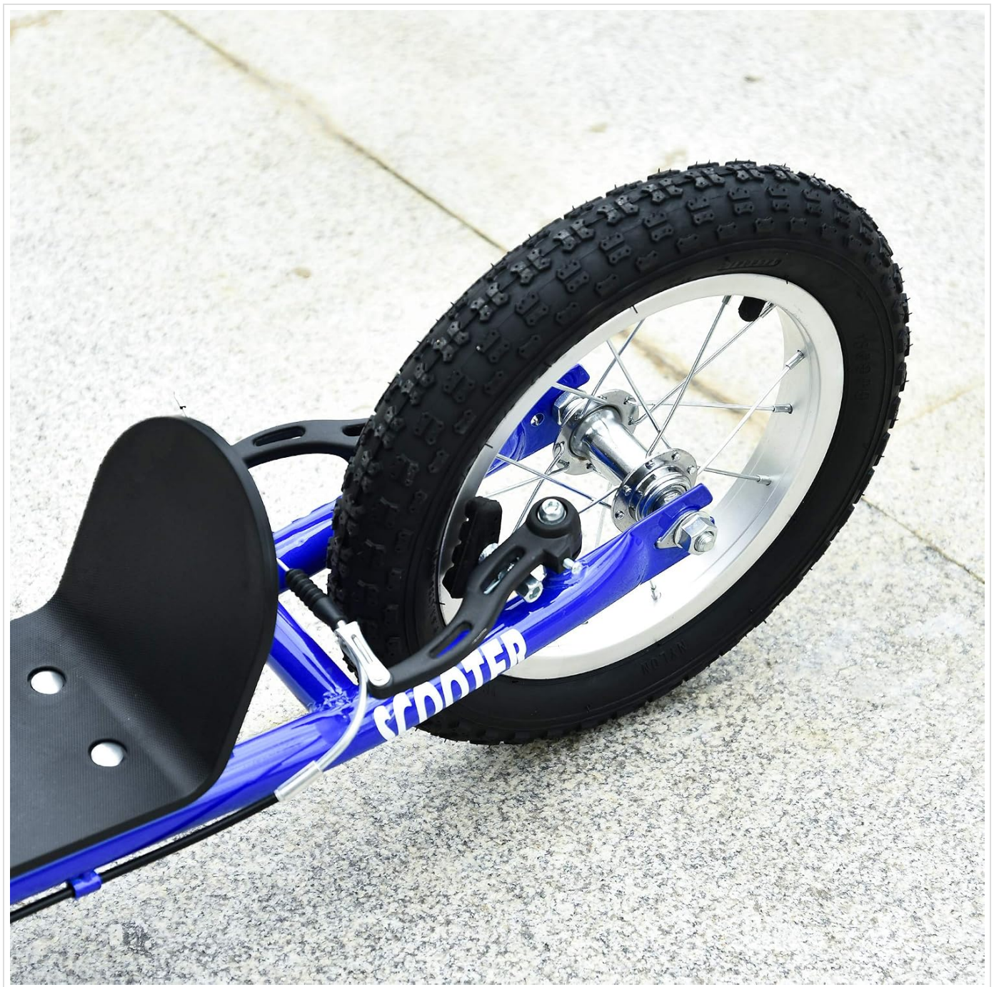
Image: Detail of the rear wheel and brake.
