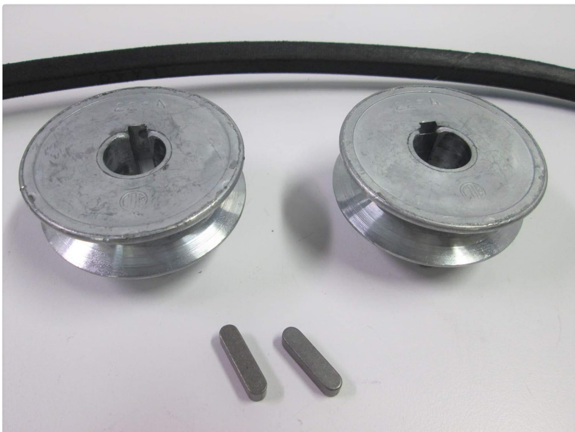
Figure 1: Complete V-Belt Kit showing the two pulleys, two keys, and the V-belt.
