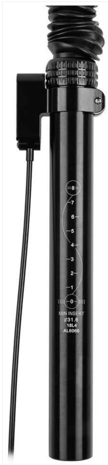
Figure 4: Close-up of the seatpost's lower tube, highlighting the "MIN INSERT" mark and measurement scale for proper installation depth.
