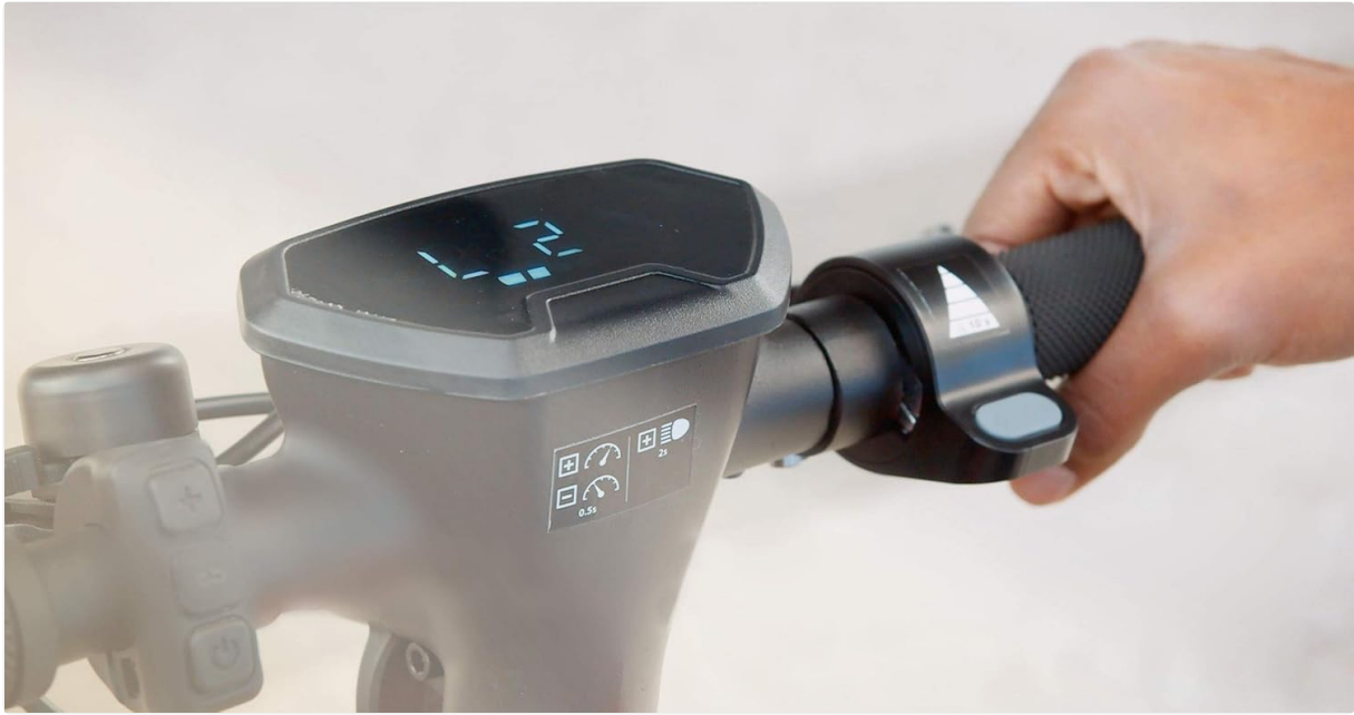
Image 3: Close-up view of the handlebar display and throttle control.
