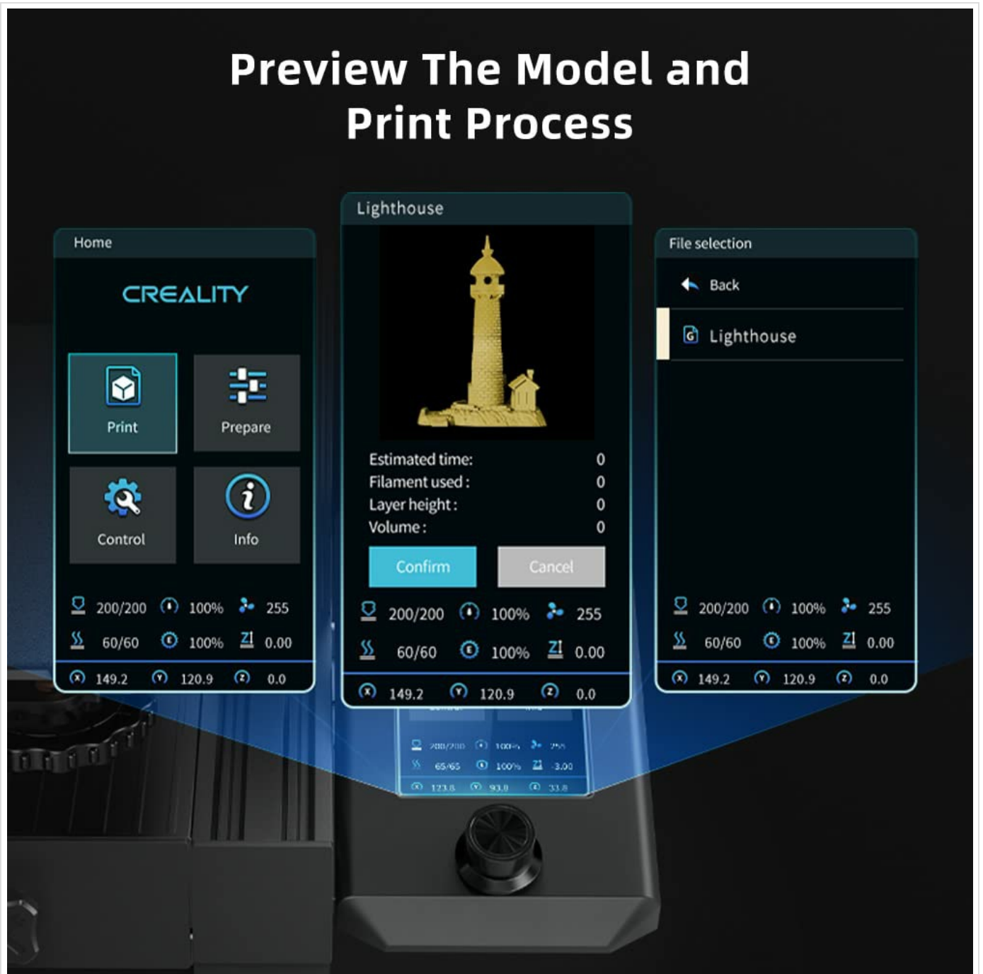
Image 5.2: The 4.3-inch user interface displaying options and a model preview screen.
