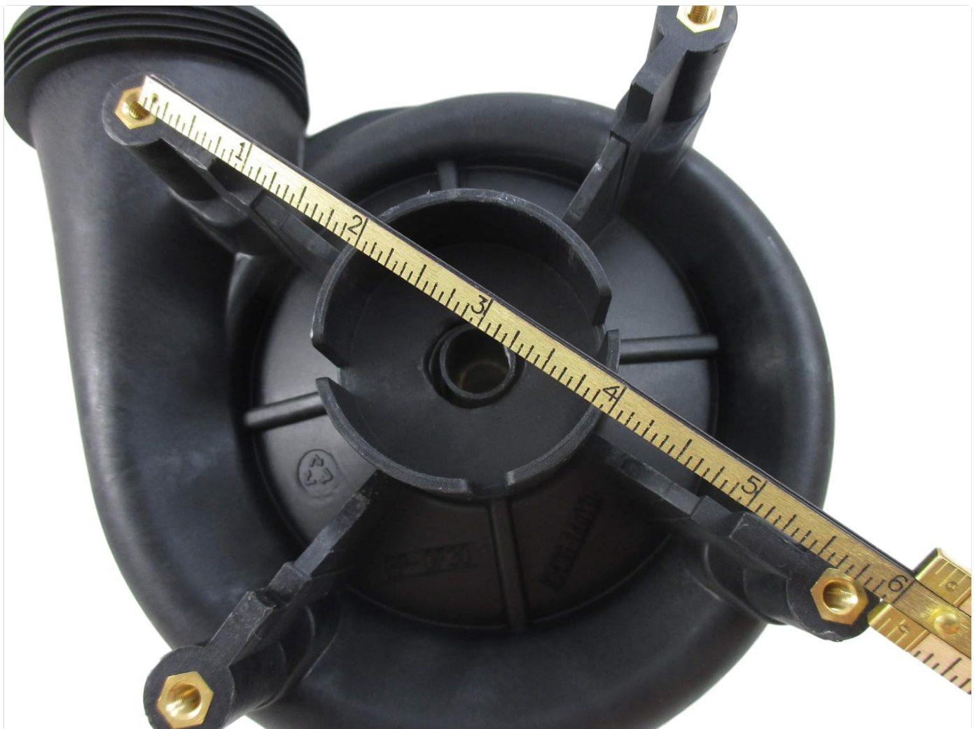
Figure 4.4: Measurement showing the 56fr frame size, which is 5 7/8 inches center-to-center on the X bolt pattern.
