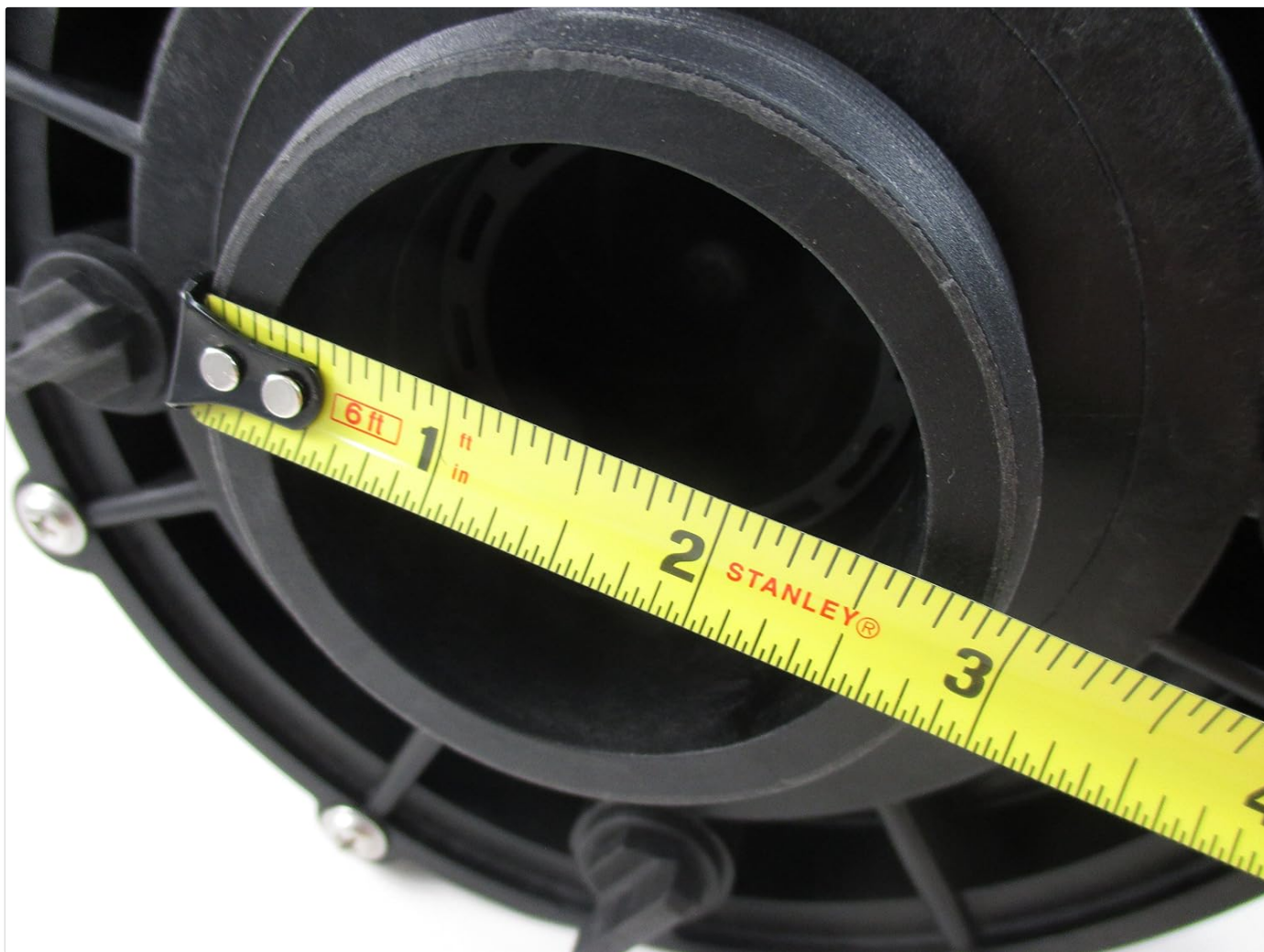
Figure 4.3: Measurement of the 2-inch inlet/outlet, which measures approximately 3 inches across the threads.
