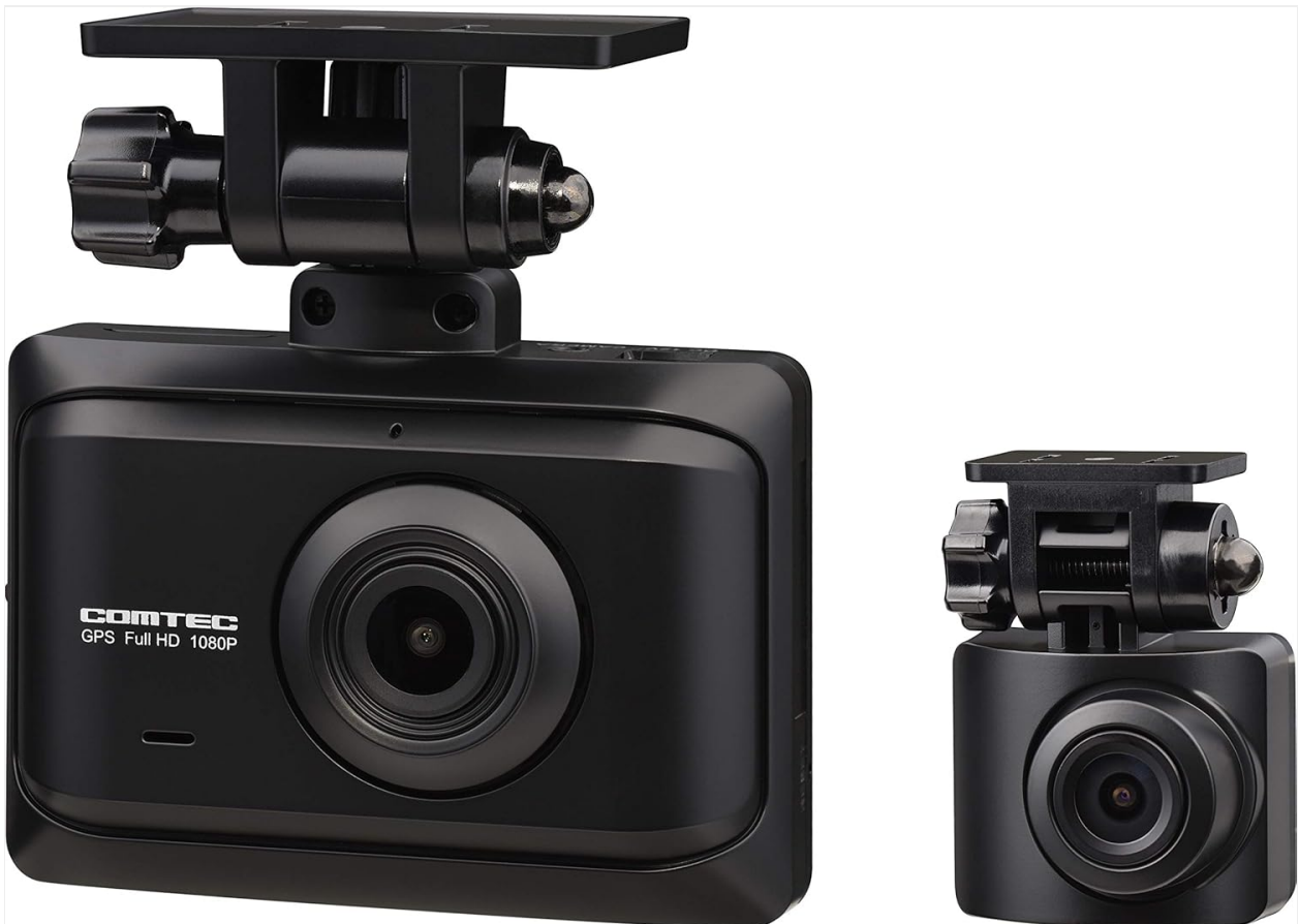
Image: The main COMTEC ZDR016 unit, showing both the front and rear camera components.
