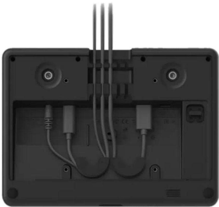
Image: Underside of the Logitech Tap Touch Controller, illustrating the cable management system and various connection ports.
