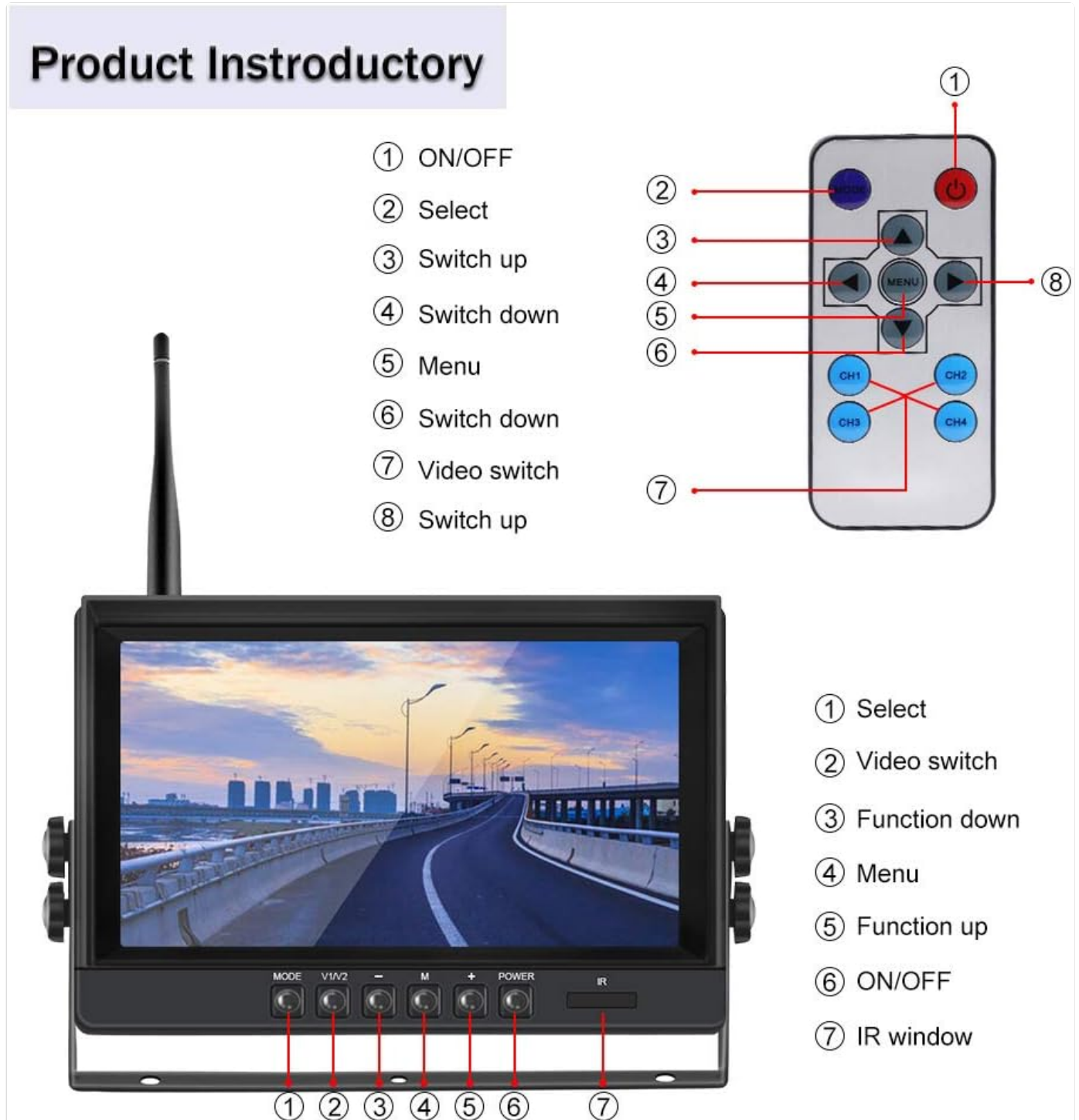
Figure 4.1: Diagram illustrating the functions of the buttons on the monitor and the corresponding remote control, including ON/OFF, Select, Switch Up/Down, Menu, and Video Switch.
