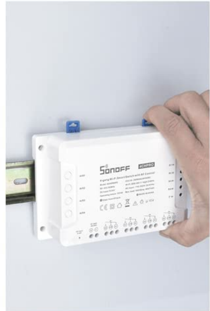
3. Press the mounting brackets until they click into place
