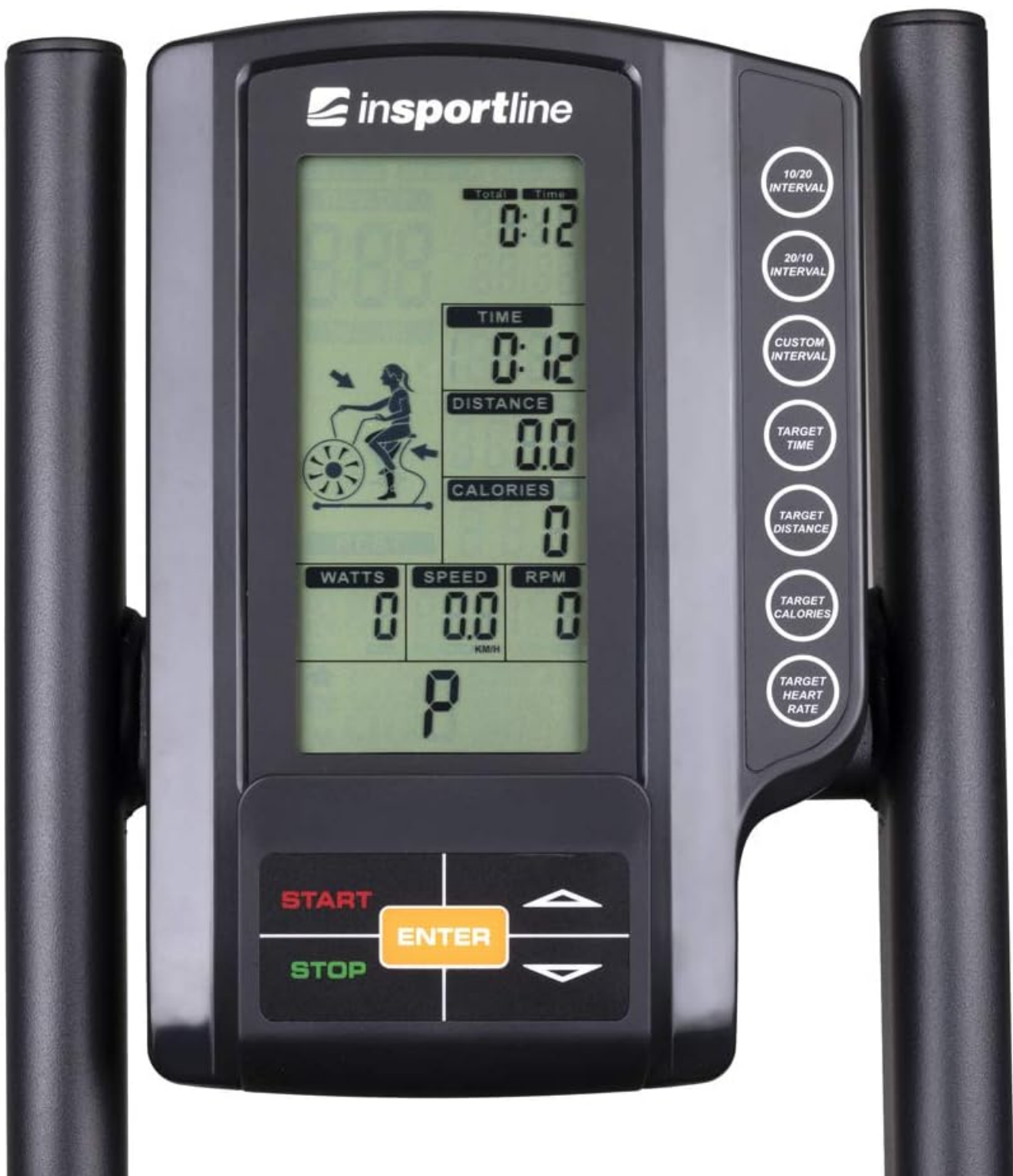
Figure 2.5: The digital console display, showing workout metrics such as time, distance, calories, watts, speed, and RPM.
