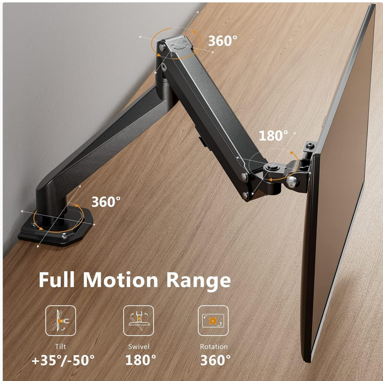
Image 6.2: Full motion range capabilities of the monitor arm.
