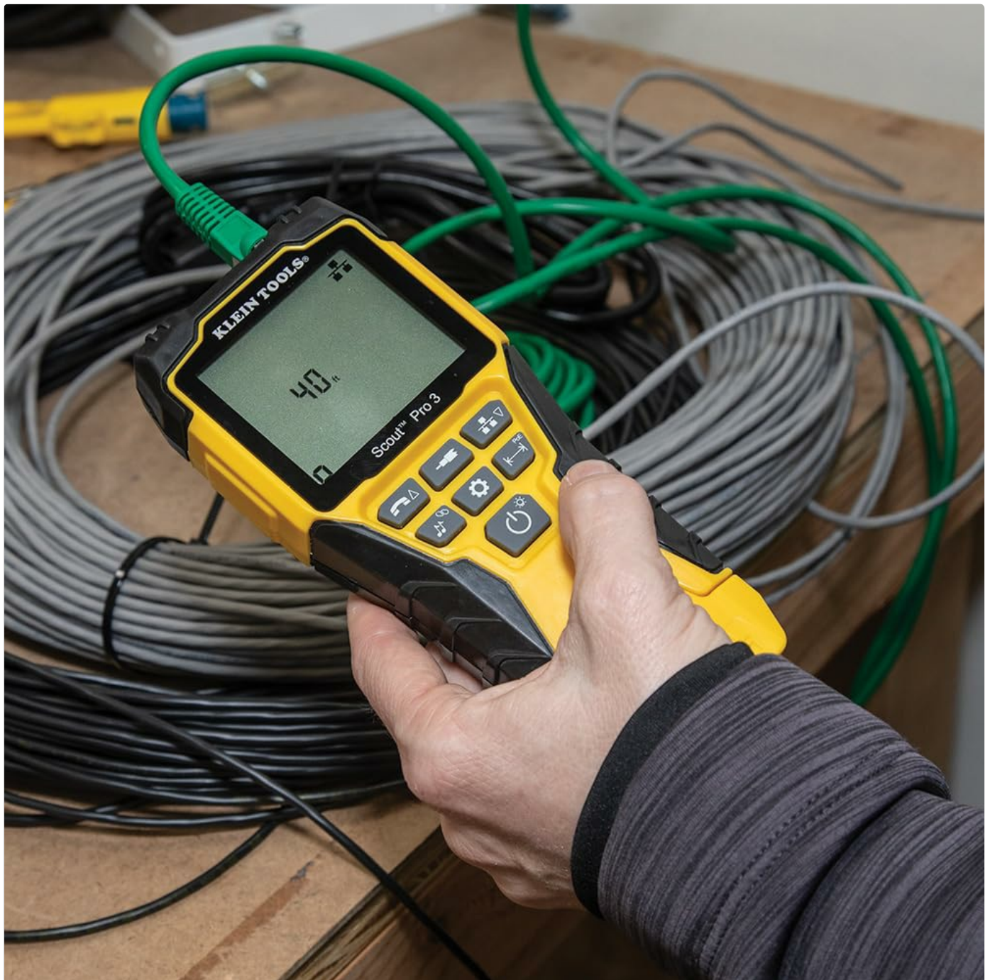
Figure 5.8: Cable length measurement display.
