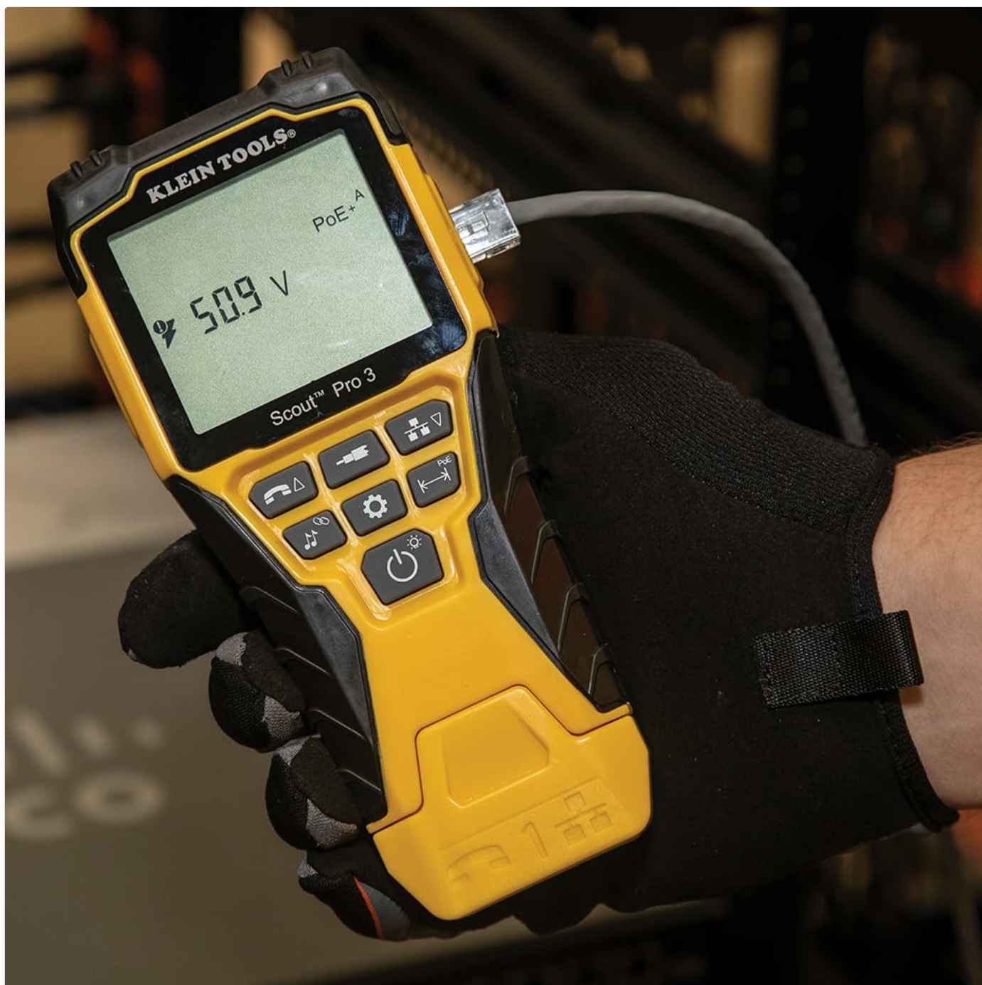
Figure 5.6: Display showing PoE voltage detection.
