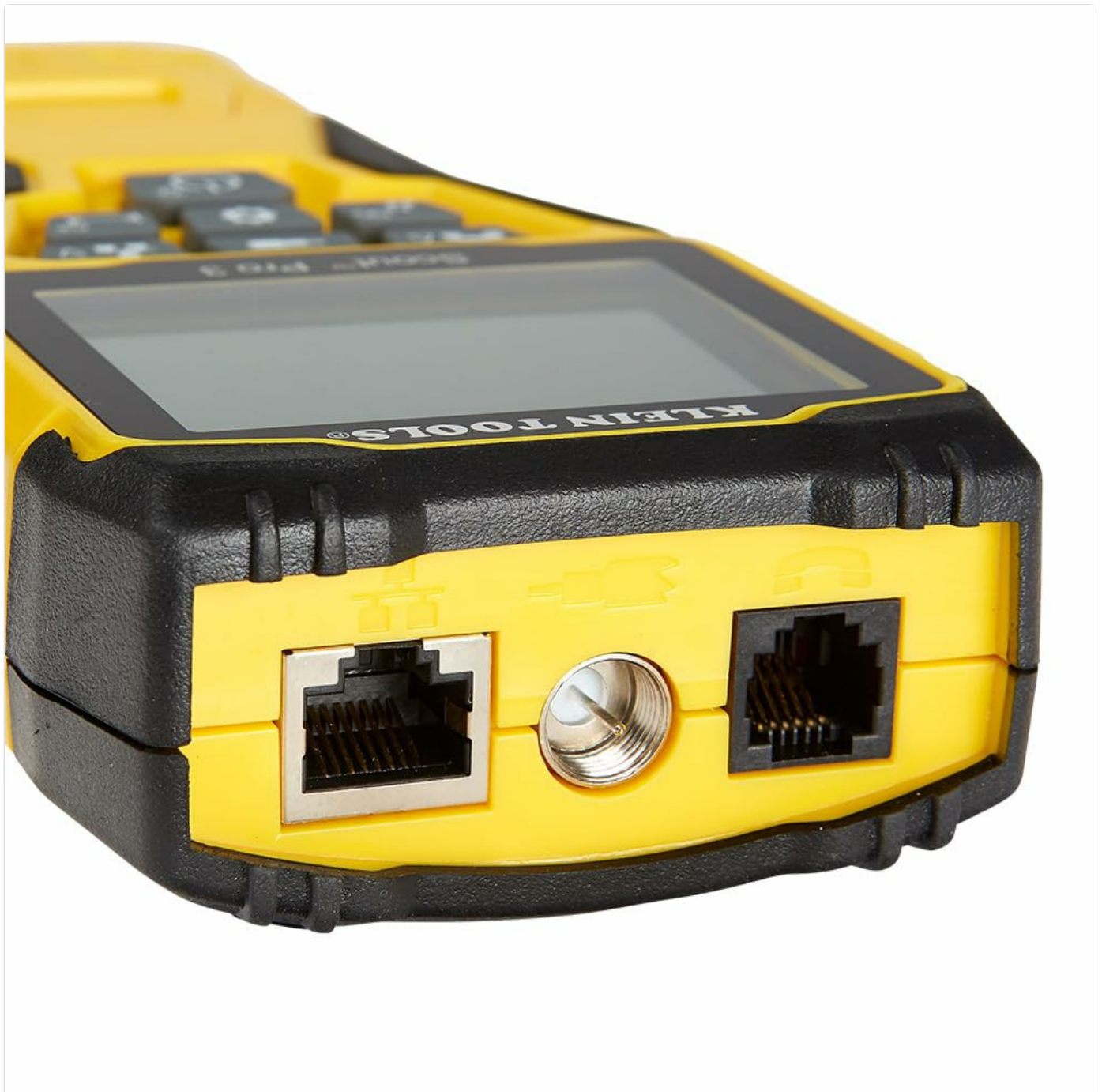
Figure 5.2: Input ports for various cable types.
