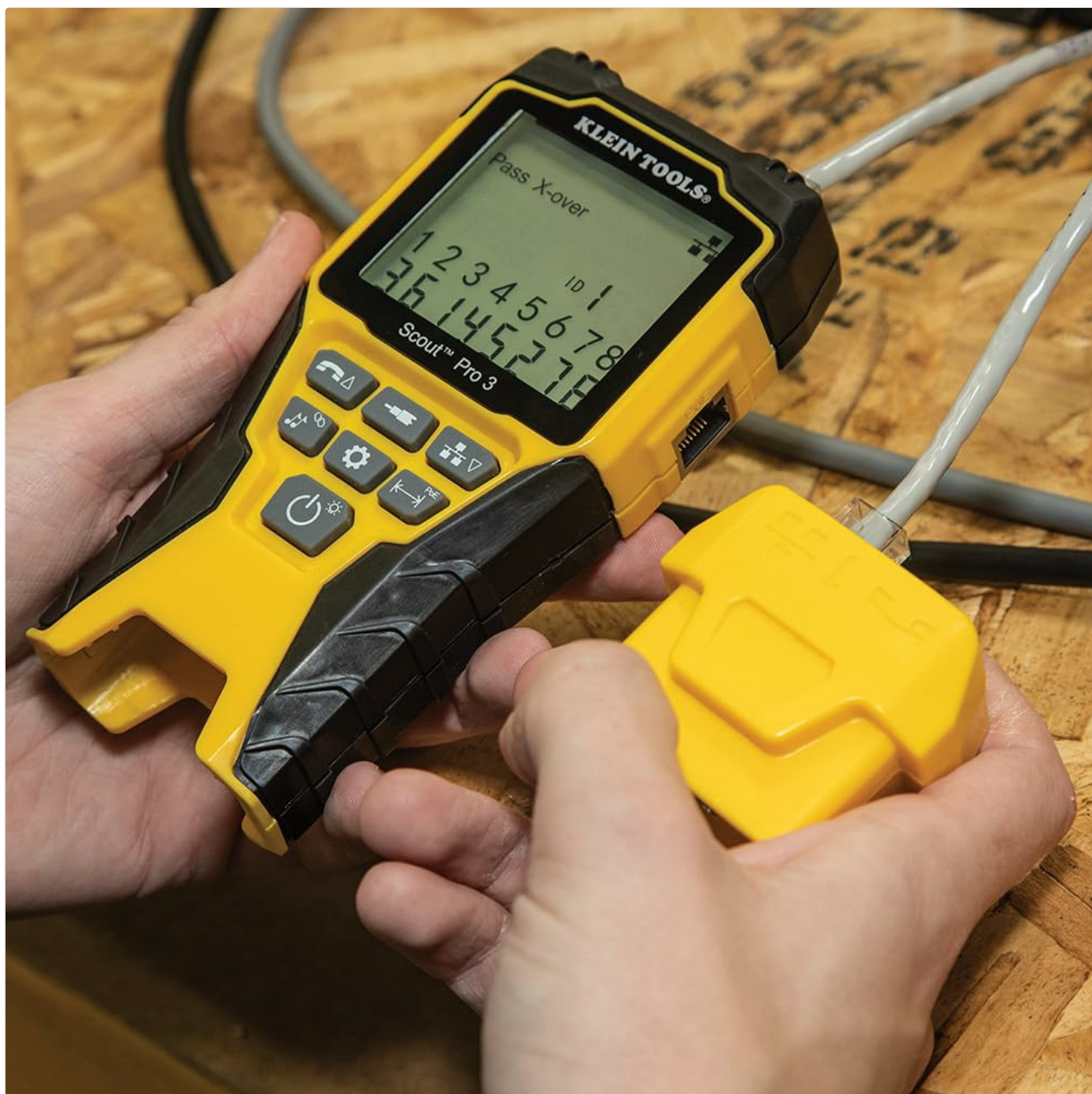
Figure 5.4: Display showing a 'Pass X-over' condition with remote ID.
