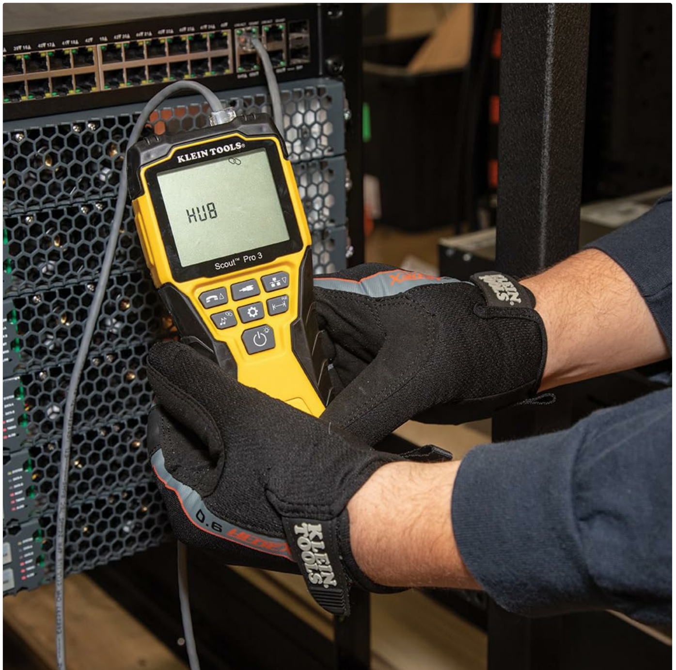
Figure 5.9: Tester in Hub Blink mode.
