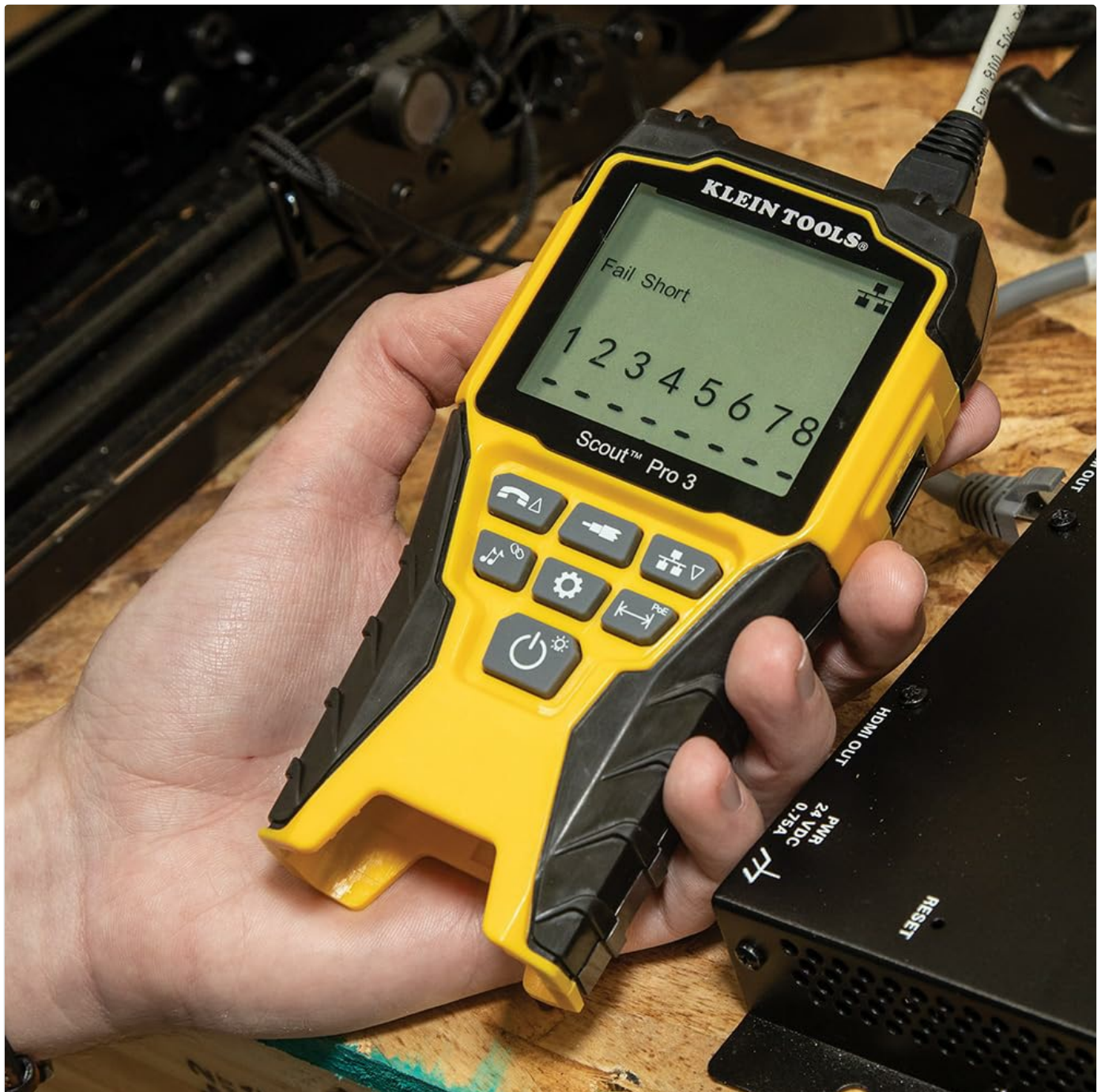
Figure 5.3: Display showing a 'Fail Short' condition.
