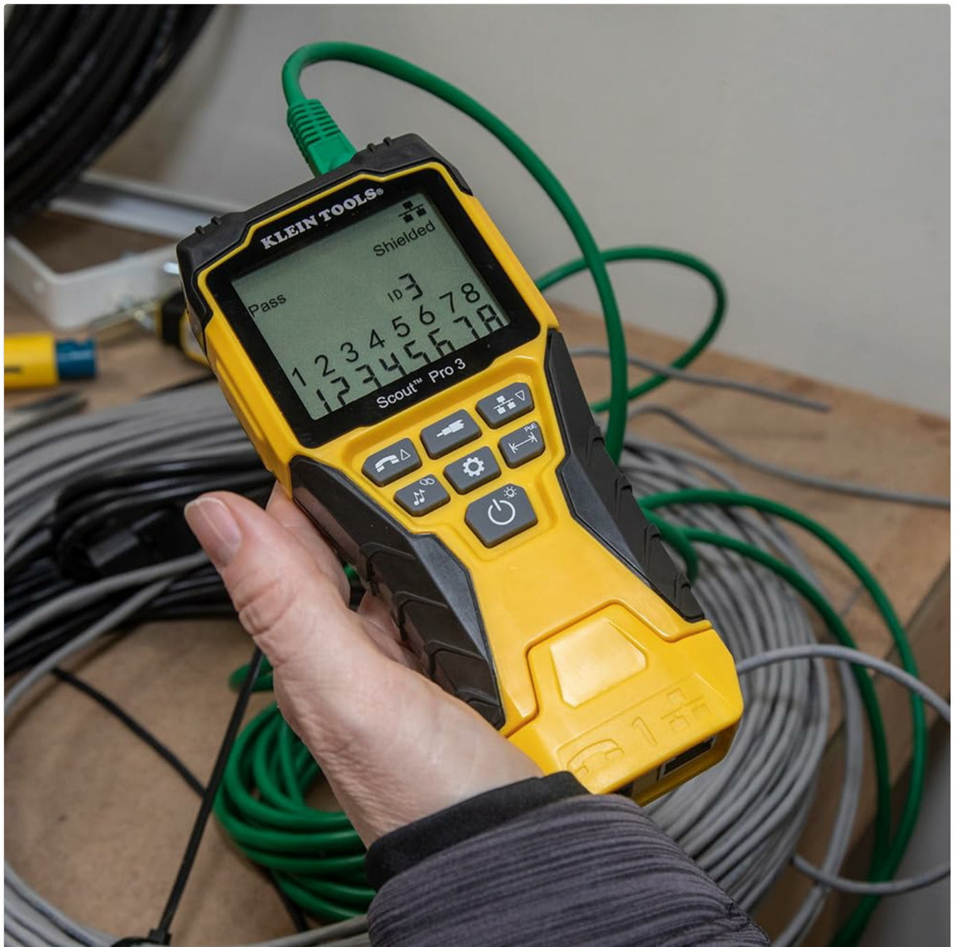
Figure 5.5: Display showing a 'Pass Shielded' condition.
