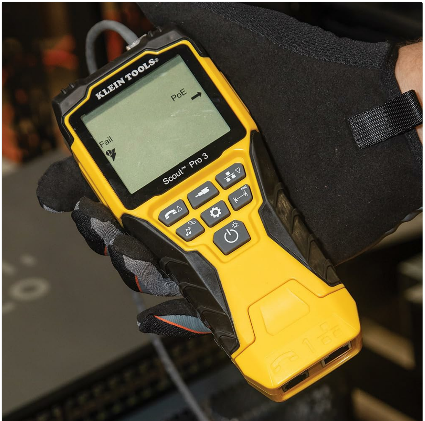
Figure 5.7: Display showing a 'Fail PoE' condition.
