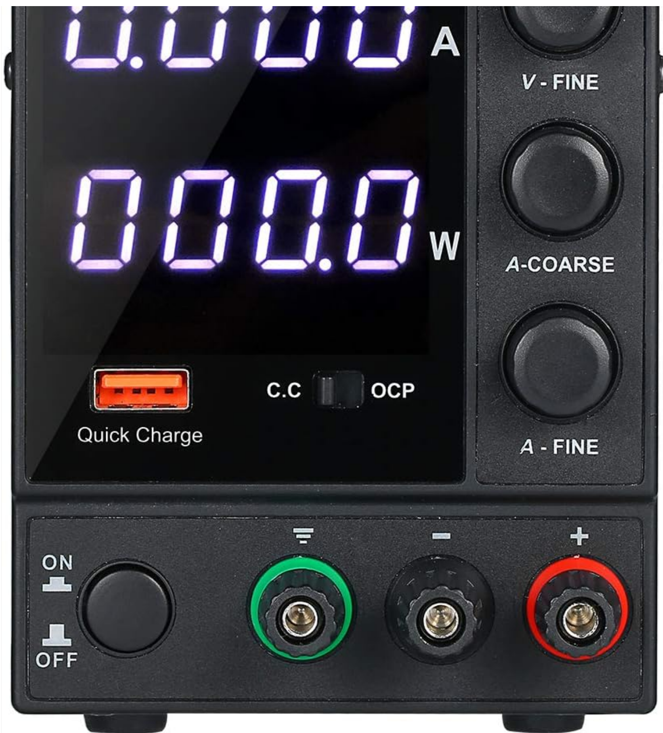
Figure 1.1: Front view of the WANPTEK DPS3010U DC Power Supply, showing the LED display and control knobs.
