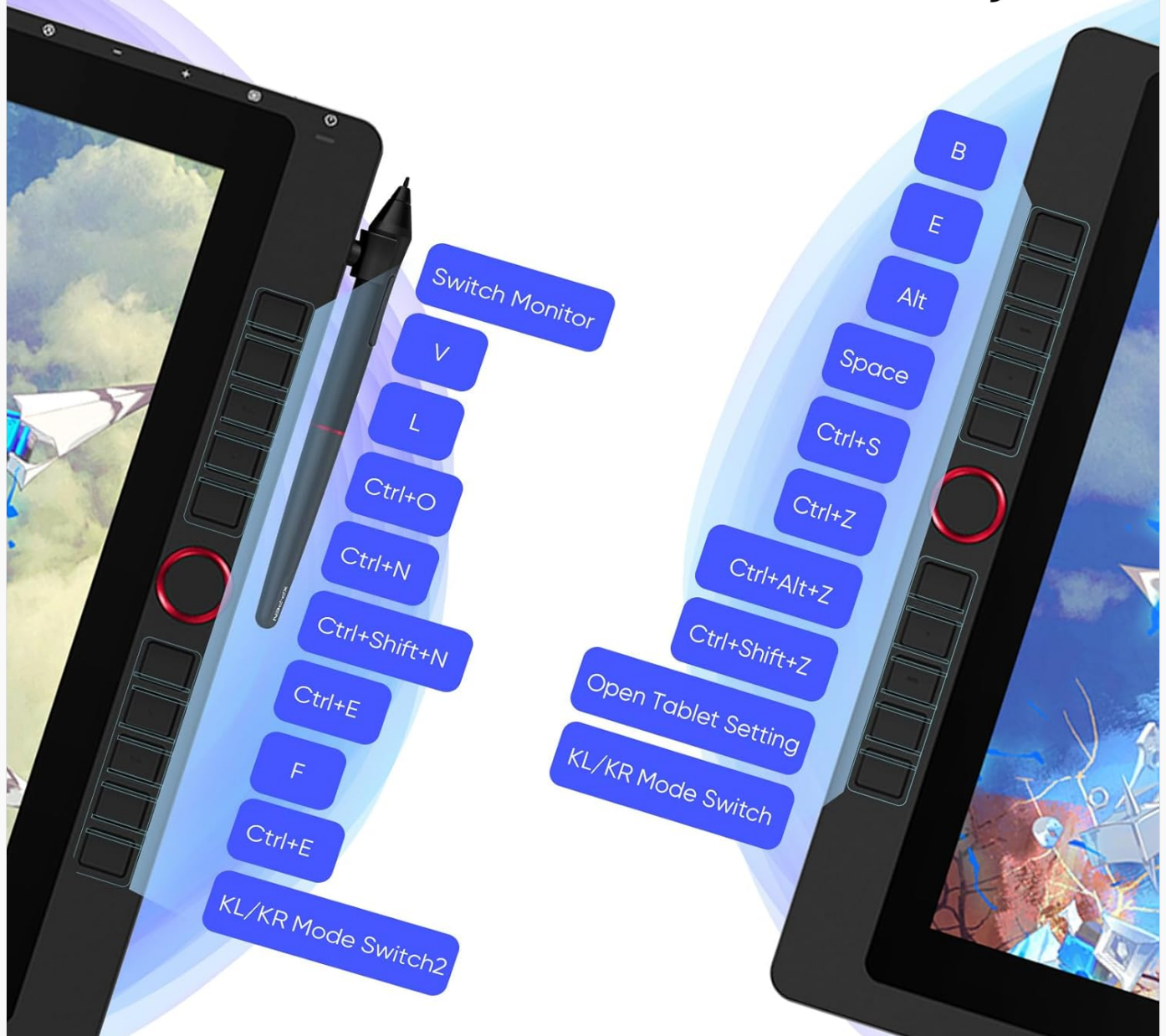
Image: Layout of the 20 customizable shortcut keys and dual red dial wheels on the Artist 24 Pro, showing examples of assigned functions.
