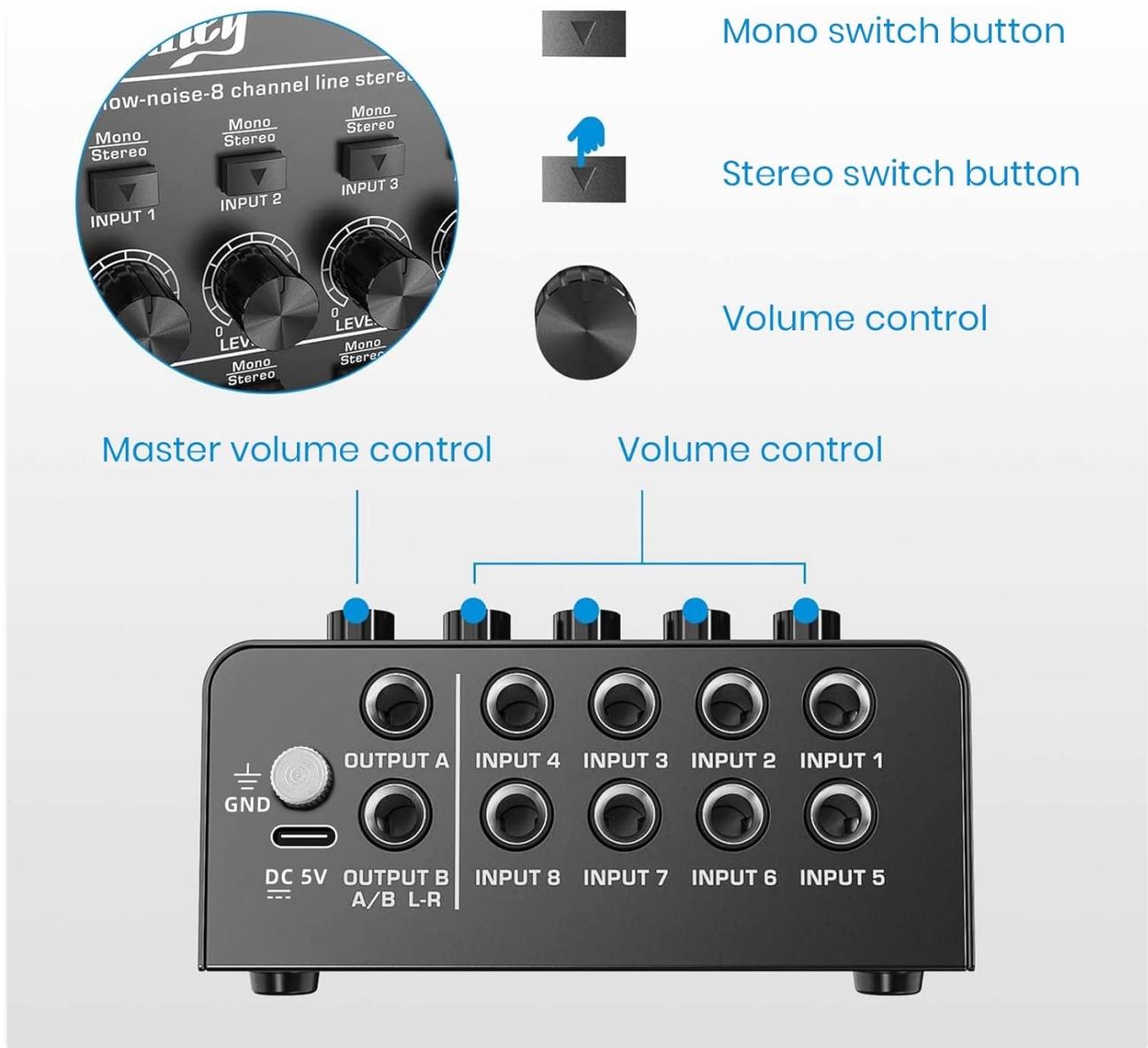
Figure 4: Control Panel Overview. Details the mono/stereo switches and individual level controls for each input.
