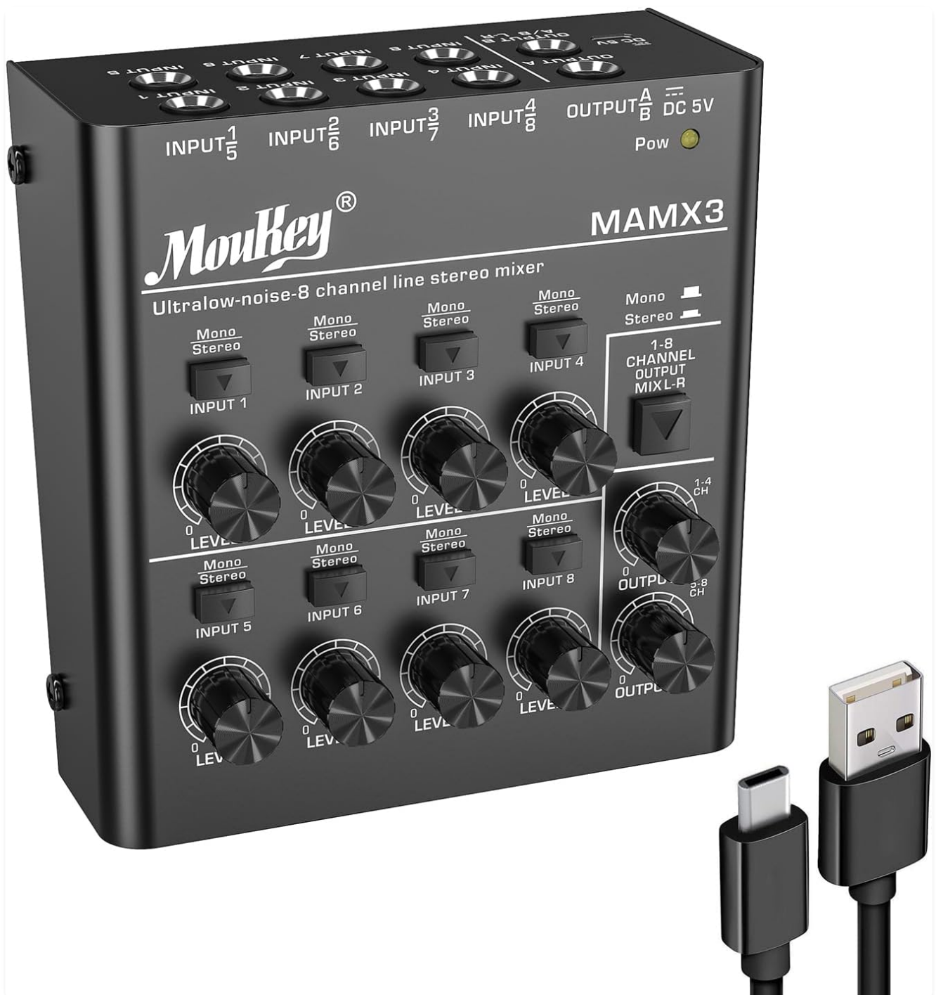
Figure 1: Moukey MAMX3 8-Channel Line Mixer. This image displays the compact design and the included USB power cable.
