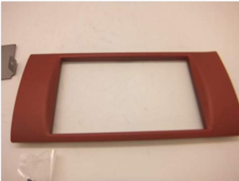
Image: Front view of the red installation panel, highlighting the central opening designed for a 2DIN audio or navigation unit.
