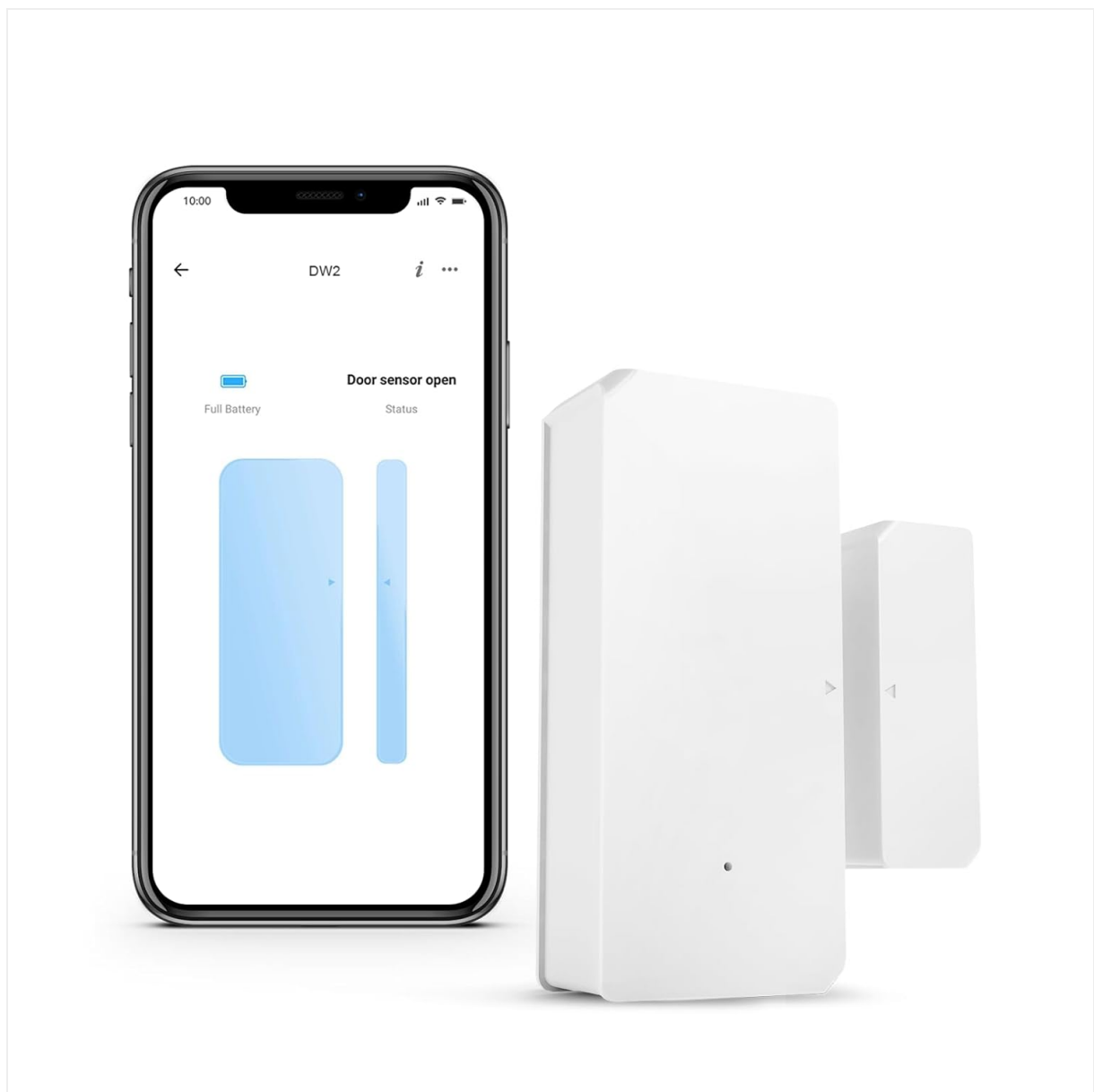
Image: The SONOFF DW2 sensor units shown alongside a smartphone displaying the eWeLink app interface, indicating the sensor's status.
