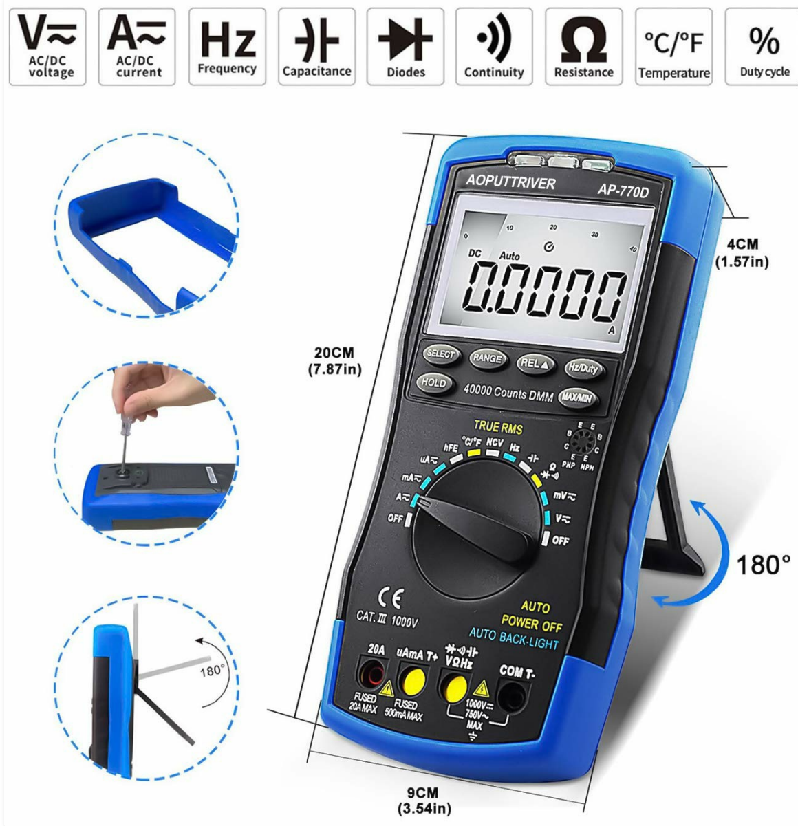
Figure 3.2: Dimensions of the AP-770D and its 180° swivel stand.
