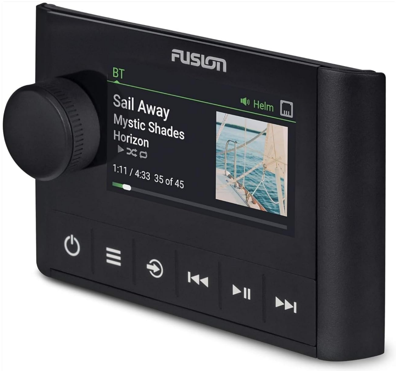
Image 4.1: Angled view of the MS-ERX400 remote. This image provides a clear perspective of the display and the arrangement of the control buttons, including the power, menu, back, and media playback buttons.
