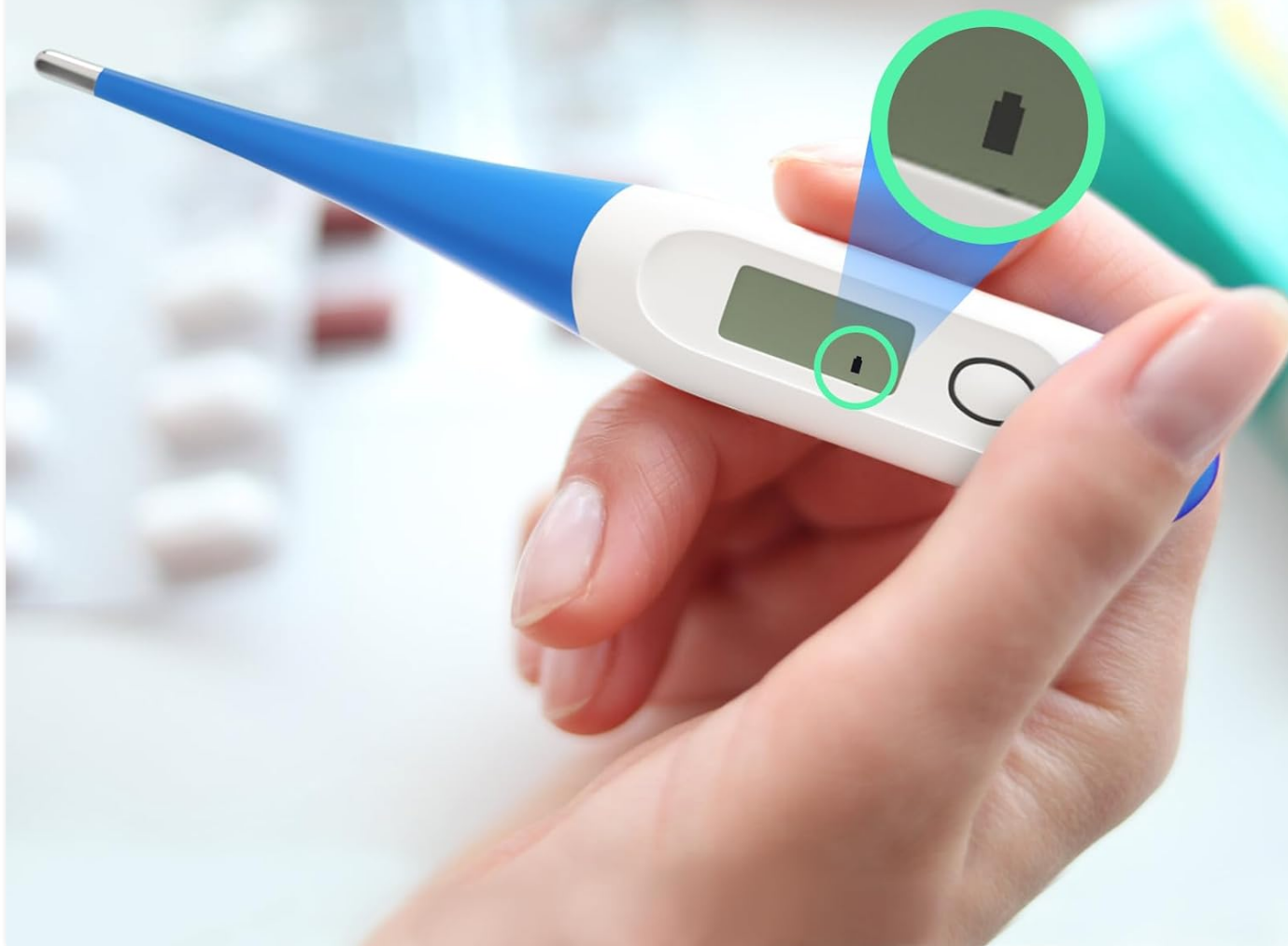
Image: A close-up of the thermometer's LCD screen, indicating a low battery with a small battery icon.
