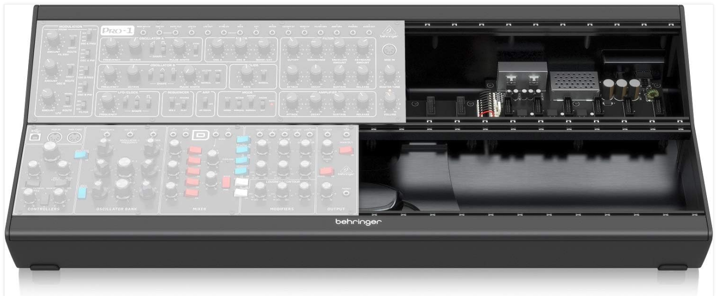
Figure 3.2: The EURORACK GO case with an example of module installation. Note the two rows of 140 HP mounting space and the internal power distribution system. Modules are secured to the rails using screws and sliding nuts.
