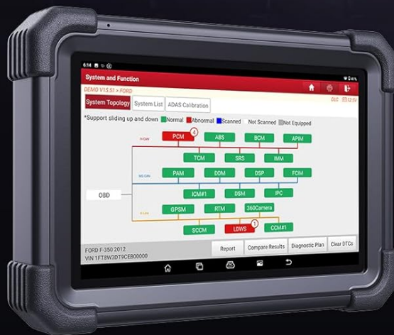
Figure 4.1: The Topology Mapping feature visually displays the system structure and communication status, aiding in quick problem identification.
