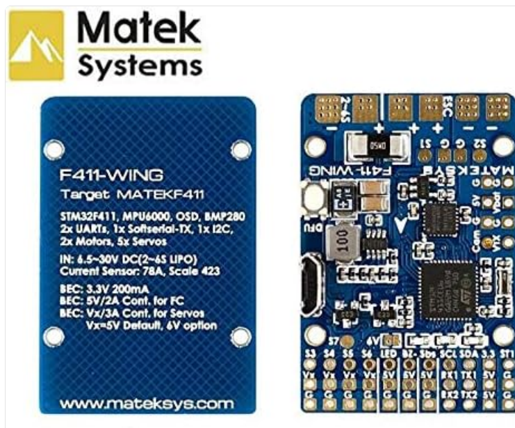
Image 2.1: Detailed views of the F411-WING flight controller, showing the top and bottom sides with component labels and specifications.
