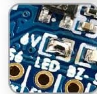
Image 4.2: Detailed board layout of the F411-WING, highlighting key components, pads, and their functions.
