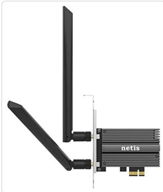
Image 1: Netis WiFi 6 AX200 PCIe card with two antennas attached, viewed from the side.
