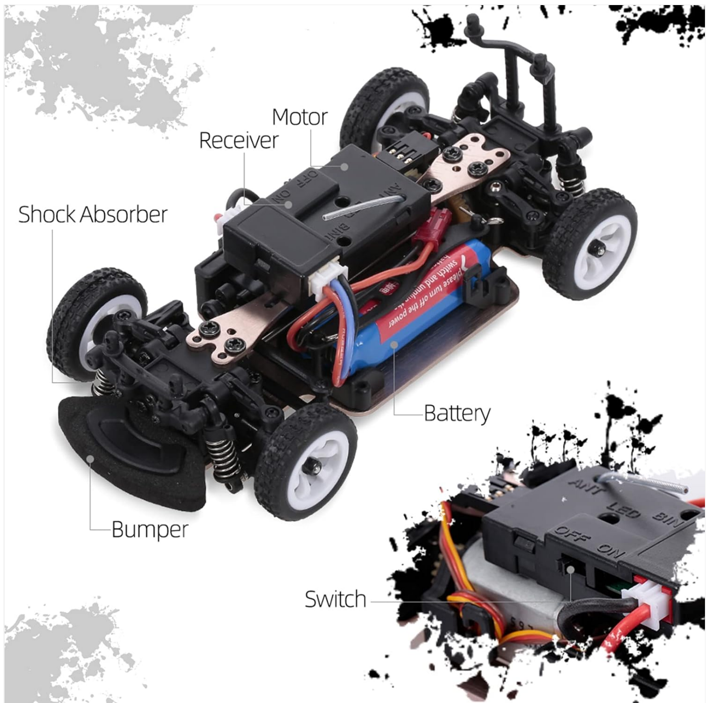
Image: An exploded view of the RC car's chassis, highlighting the battery, motor, receiver, shock absorbers, bumper, and switch.
