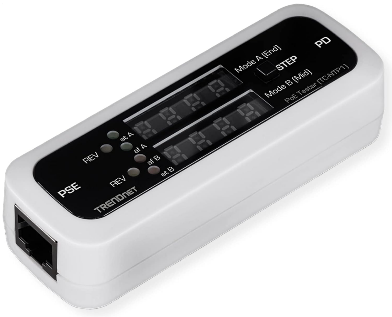
Figure 4.1: Angled view of the TRENDnet TC-NTP1 Inline PoE Tester, showing the display and ports.
