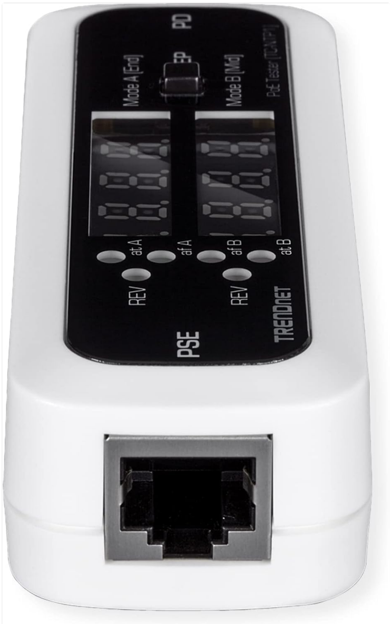
Figure 4.3: Front view of the TC-NTP1, showing the PSE (Power Sourcing Equipment) Gigabit Ethernet port.
