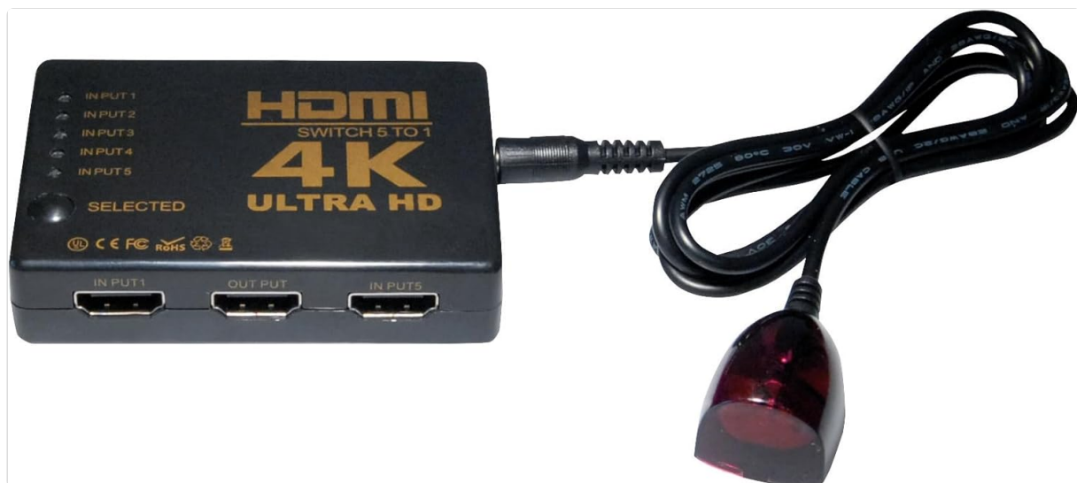
Figure 4.1: HDMI switch with IR receiver and USB power cable connected.
