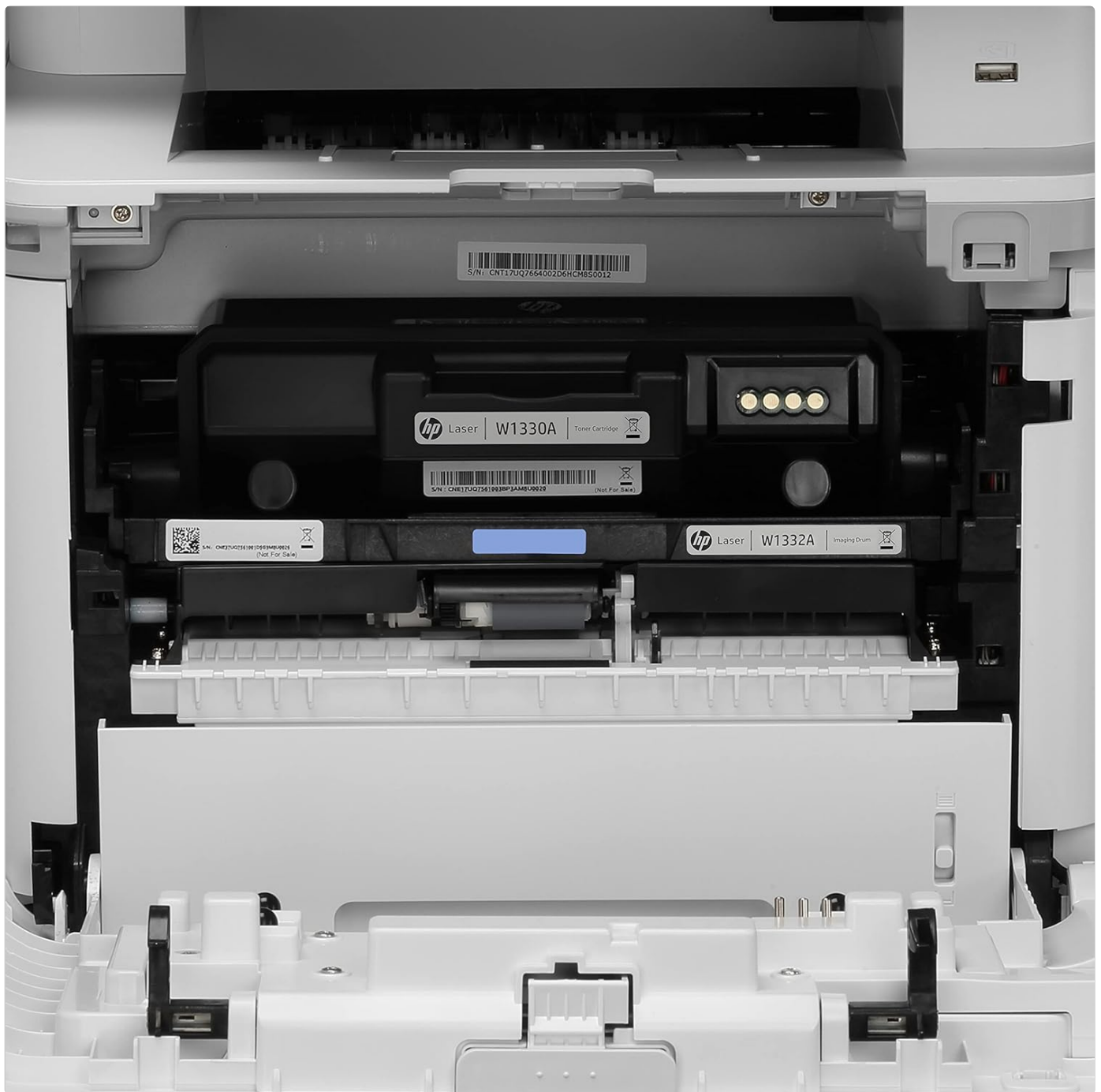
Figure 4: Toner cartridge installation area with an HP W1330A cartridge visible.
