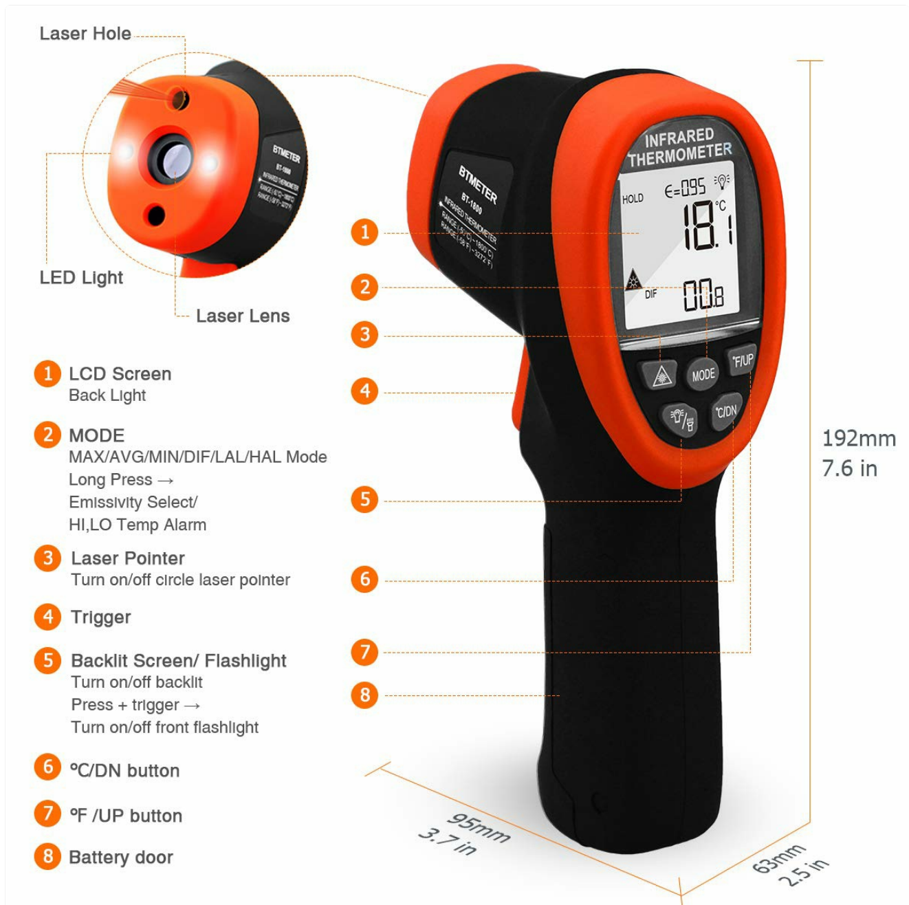
Figure 2: Key components and controls of the BT-1800 Infrared Thermometer.
