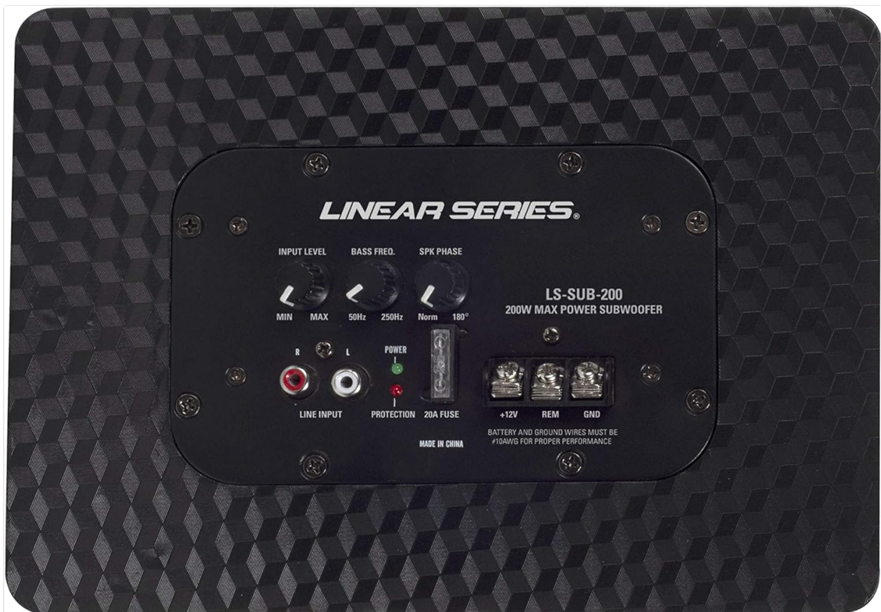
Image 4.1: Close-up view of the control panel on the Magnadyne LS-SUB-200 subwoofer, showing input level, bass frequency, speaker phase controls, RCA inputs, power/protect LED, fuse, and power terminals.
