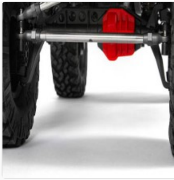
Image: A close-up of the robust suspension links and portal axle system of the Axial SCX10 III, designed for extreme articulation.
