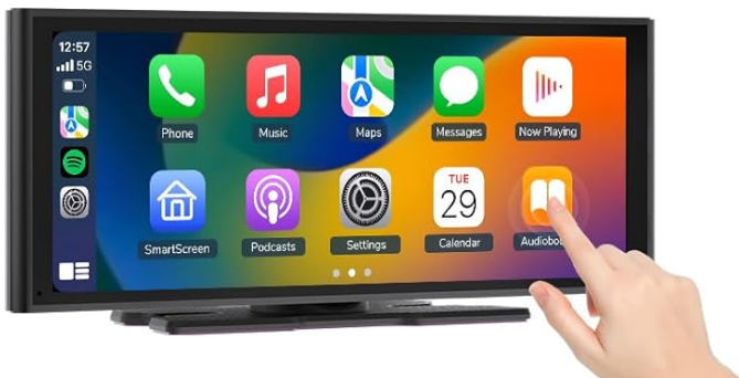
Figure 6: Highlights the 9.33-inch IPS display with 1600x600 resolution, showcasing its vibrant colors and responsive capacitive touchscreen. It also shows the detachable screen feature.
