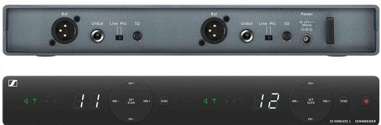
Image: Rear panel of the EM-XSW 1 receiver, displaying balanced XLR outputs, unbalanced 1/4" jack outputs, and power input.
