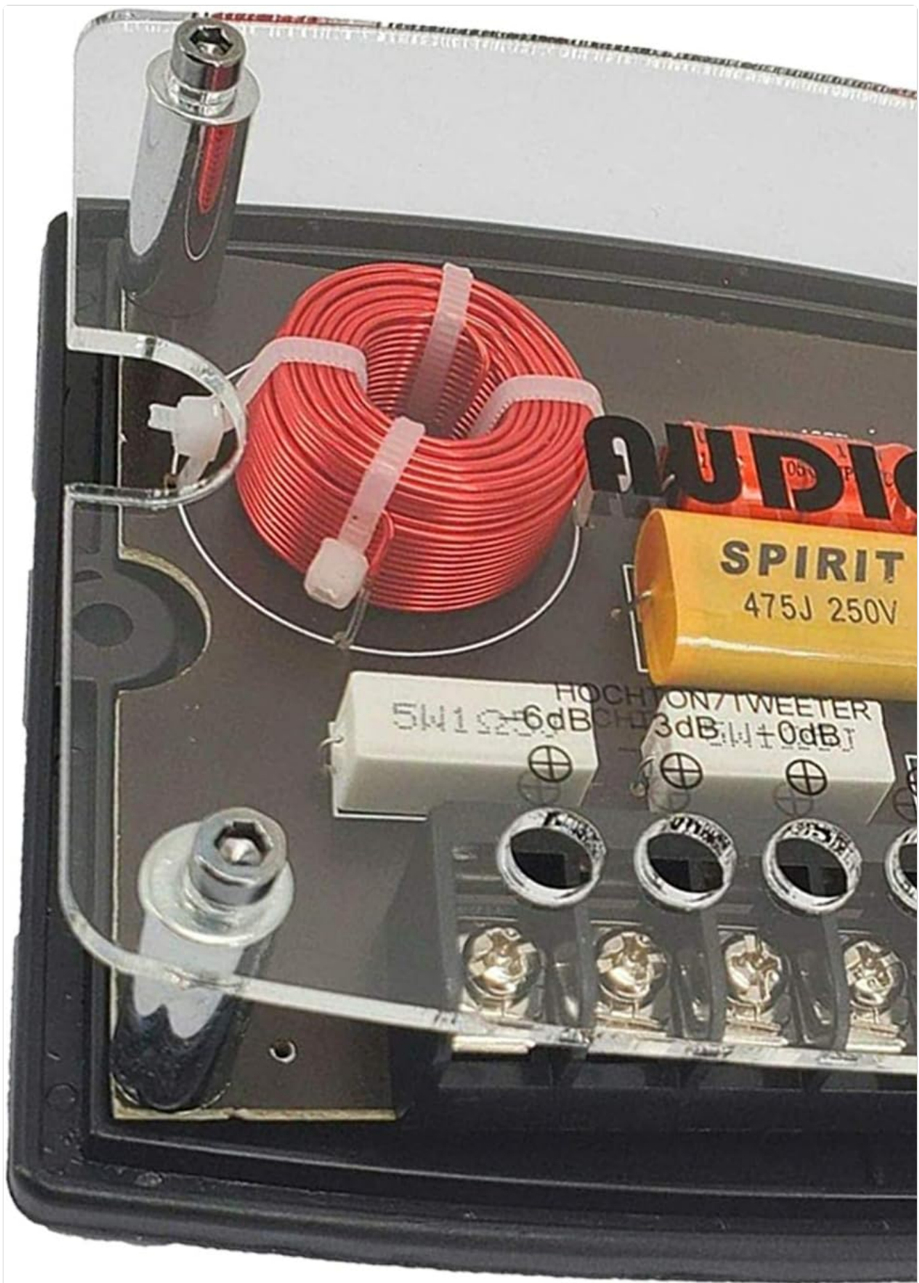
Image 1: Close-up view of the Audiotek CX4 passive crossover network, showing the input, woofer, and tweeter terminals. The transparent plexiglass cover allows visibility of the internal components, including the red coils and yellow capacitor.
