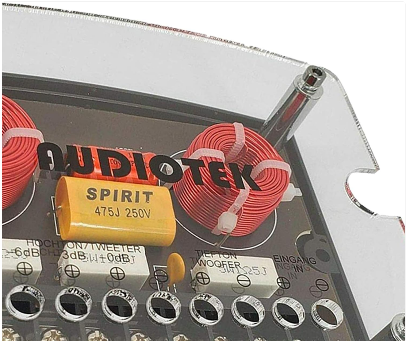
Image 2: Detailed view of the Audiotek CX4 crossover, highlighting the tweeter level adjustment jumpers (0dB, -3dB, -6dB) and the capacitor.
