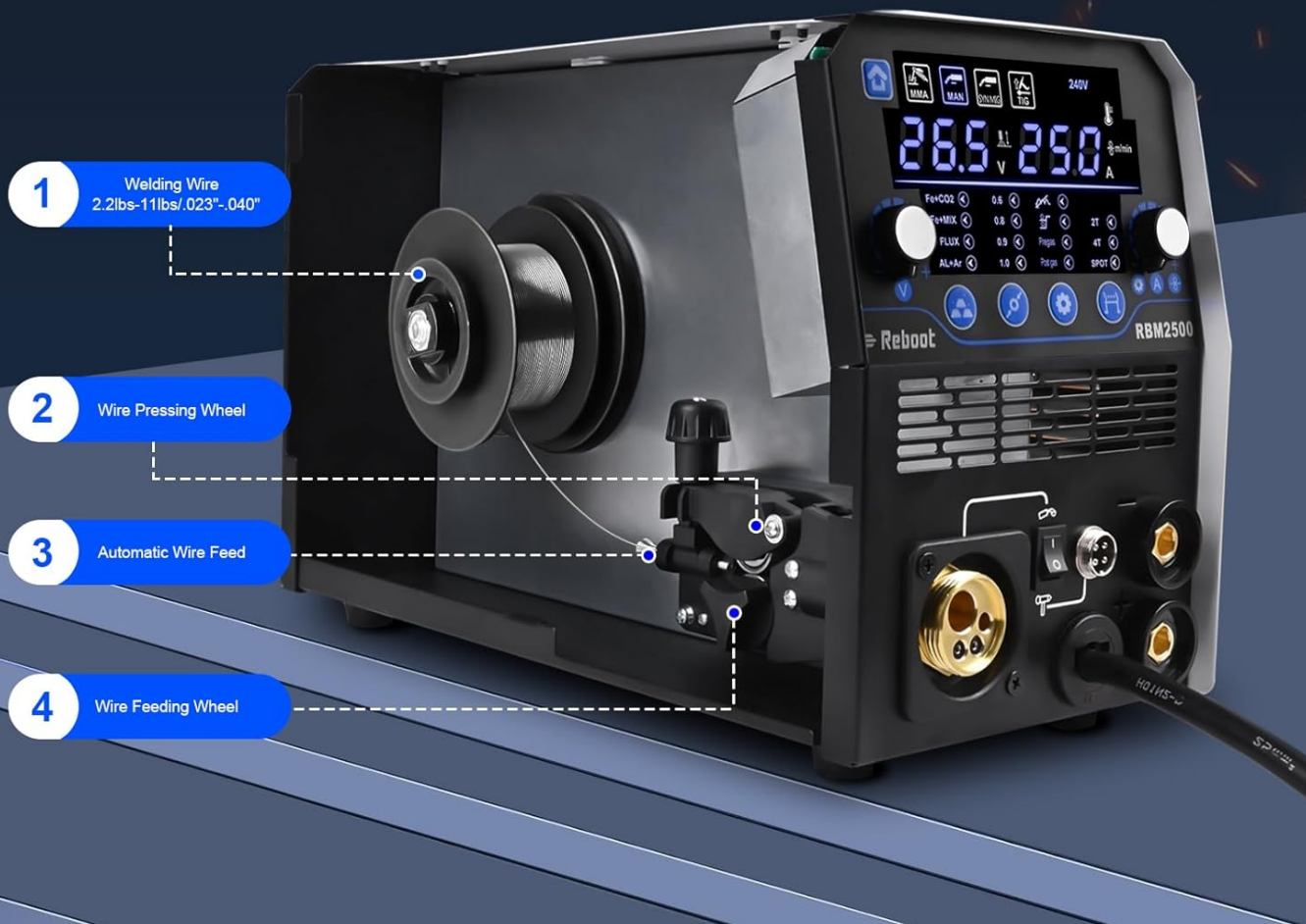
Figure 4.1: Wire Feed Structure. 1. Welding Wire, 2. Wire Pressing Wheel, 3. Automatic Wire Feed, 4. Wire Feeding Wheel.
