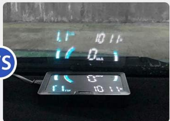
Can directly see the LED panel, affect driving.
