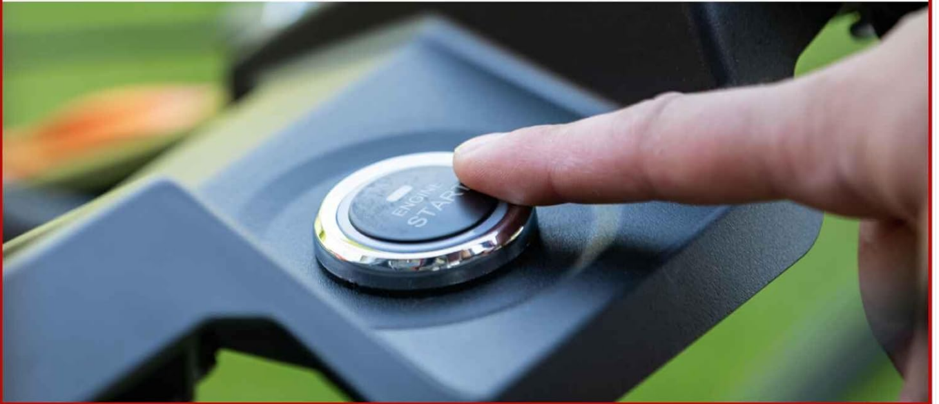
Image: Close-up of the electric start button, highlighting the convenience of the hybrid start system which eliminates the need for choking or priming.
