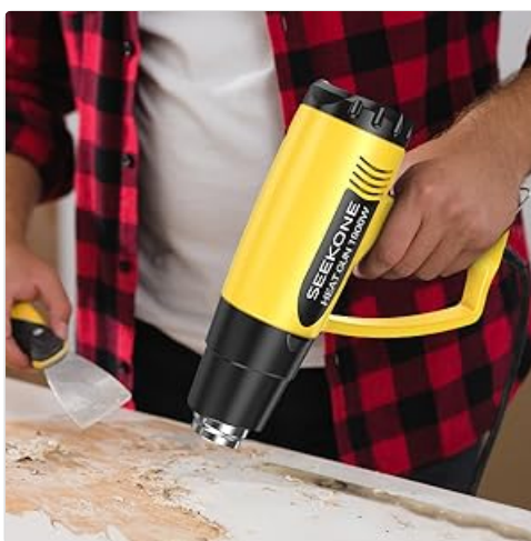
Image 6.4: Example of using the heat gun for paint removal from a wooden surface.
