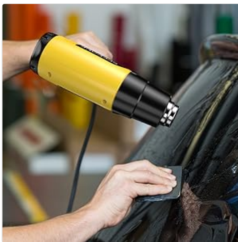
Image 6.3: Example of using the heat gun for shrinking applications, such as window film.
