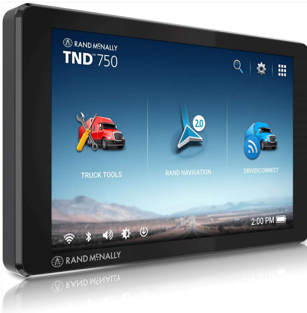
Figure 2.1: Rand McNally TND 750 GPS Unit. The main screen displays options for Truck Tools, Rand Navigation, and DriverConnect.
