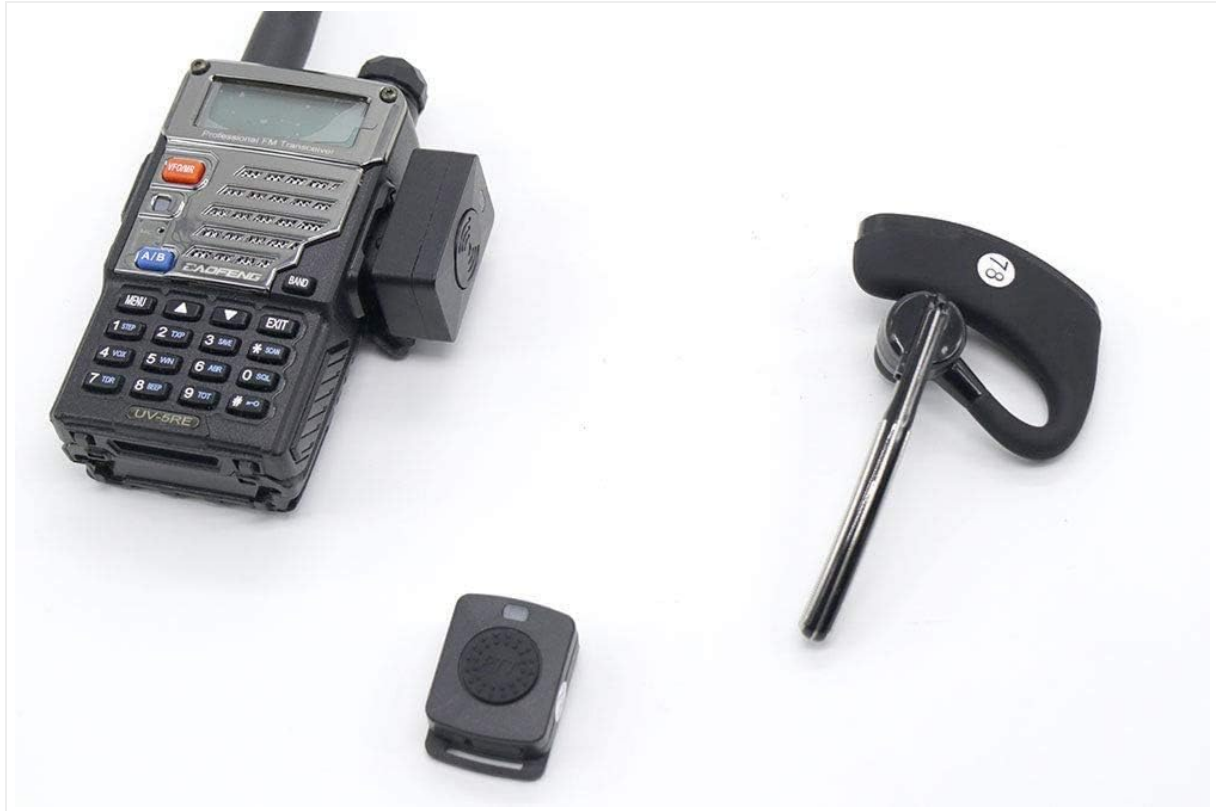
Image: A two-way radio (Baofeng UV-5RE) with the wireless adapter attached, alongside the Bluetooth headset and wireless PTT button, demonstrating a complete setup.
