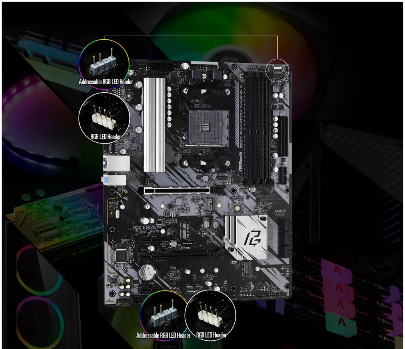
Image: The motherboard includes both 4-pin RGB LED headers and 3-pin Addressable RGB LED headers for customizable lighting.
