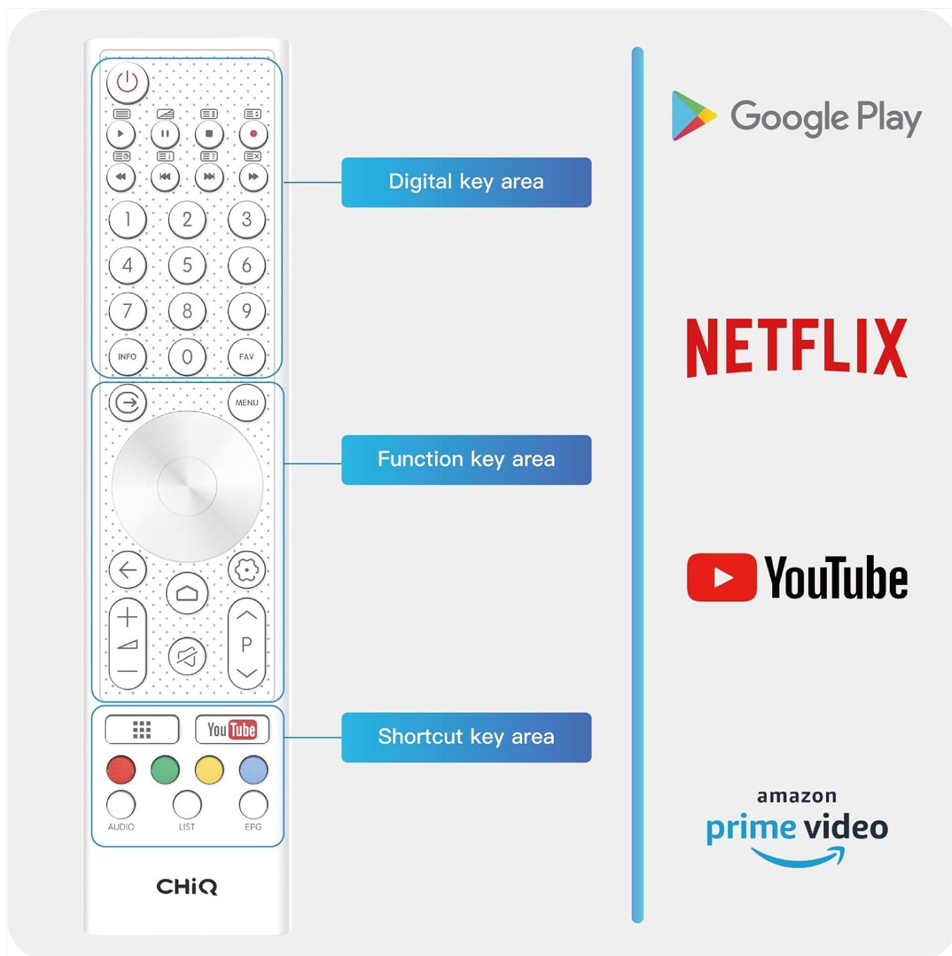
Figure 3: Layout of the CHiQ Smart TV remote control, showing digital, function, and shortcut key areas.
