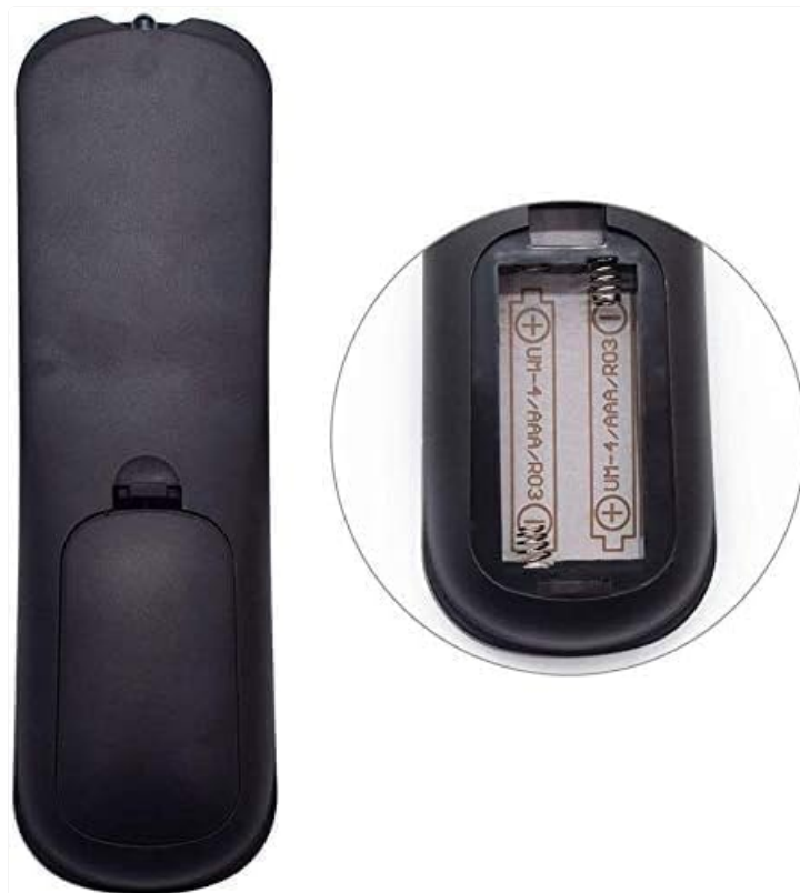
Image 2.1: Rear view of the remote control showing the battery compartment.
