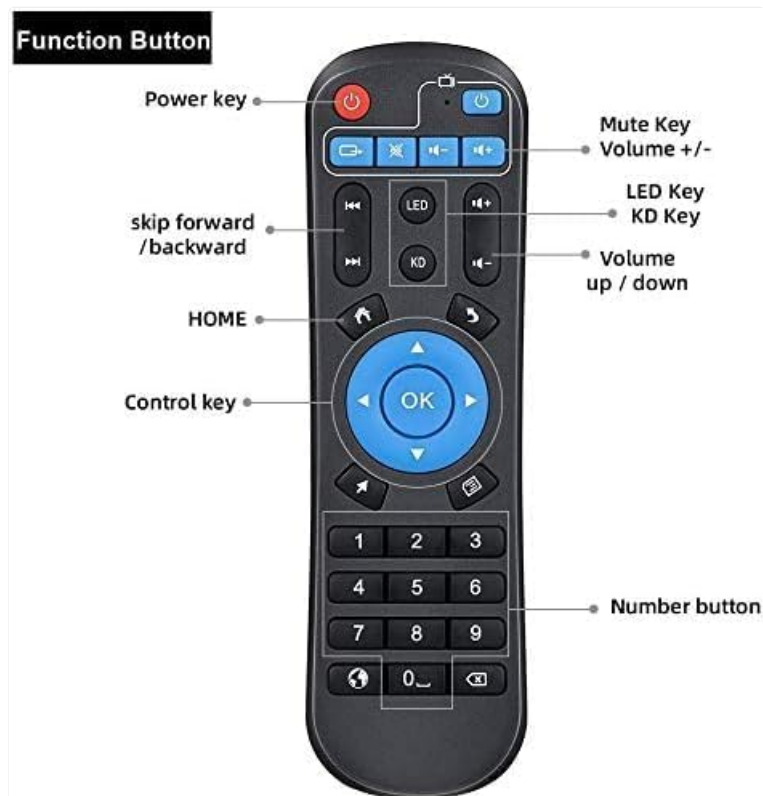
Image 3.1: Diagram illustrating the function of each button on the remote control.
