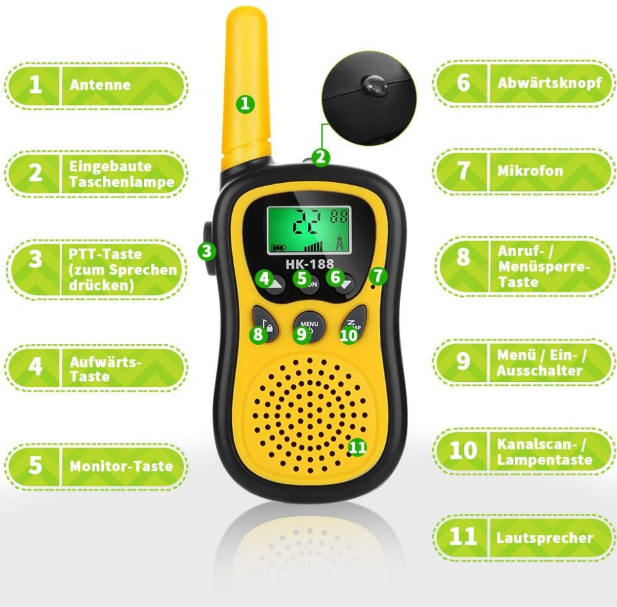
Image: Labeled diagram showing the various components of the walkie-talkie.
