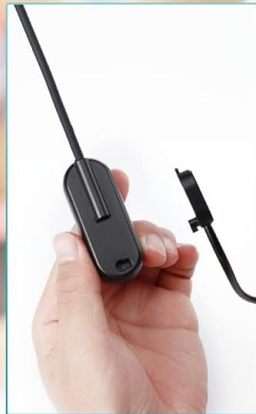
2. Bump on the head bracket facing right to the slot on the transmitter.
