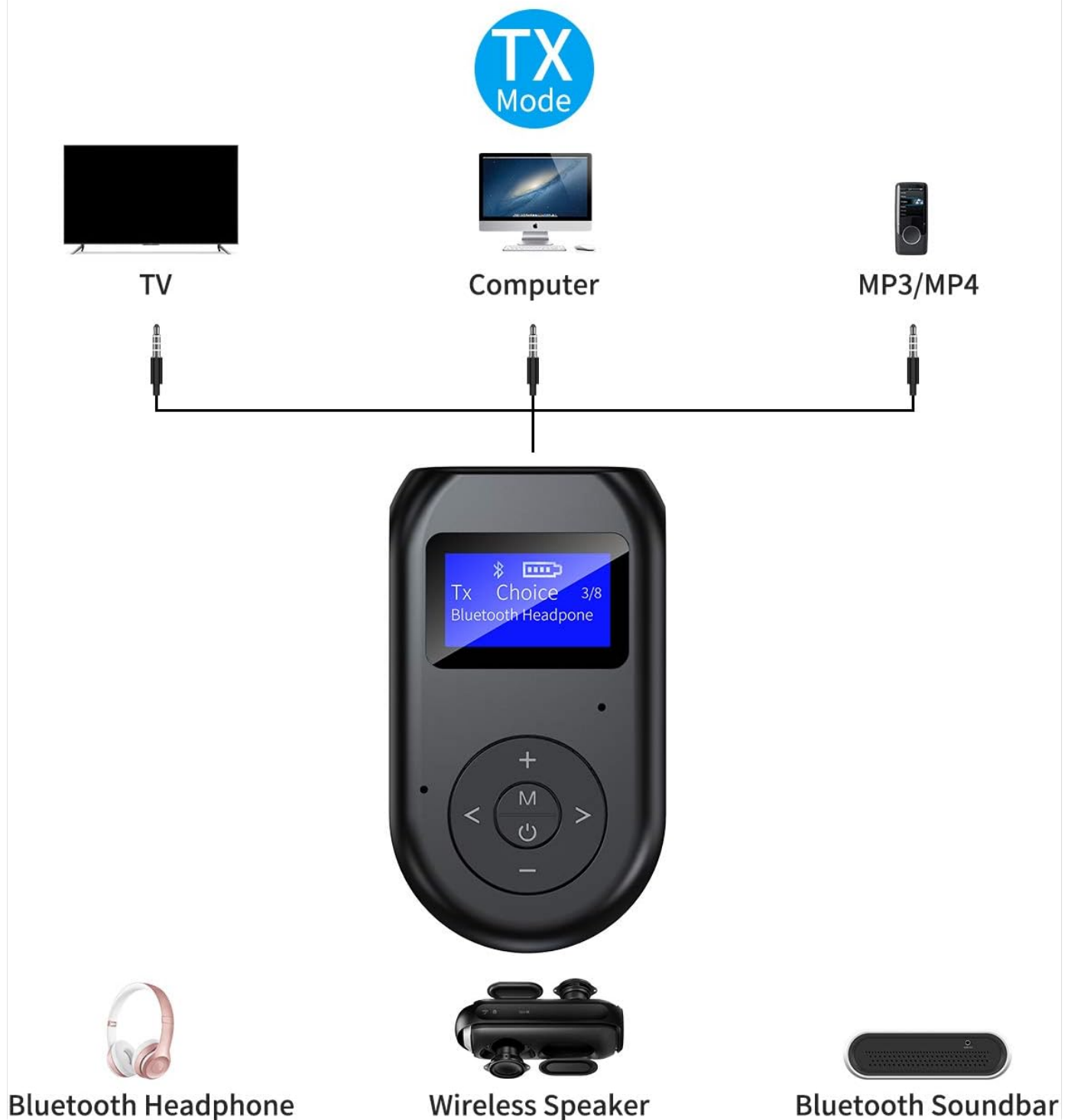
Figure 5.3: Transmitter (TX) Mode Connection Diagram
