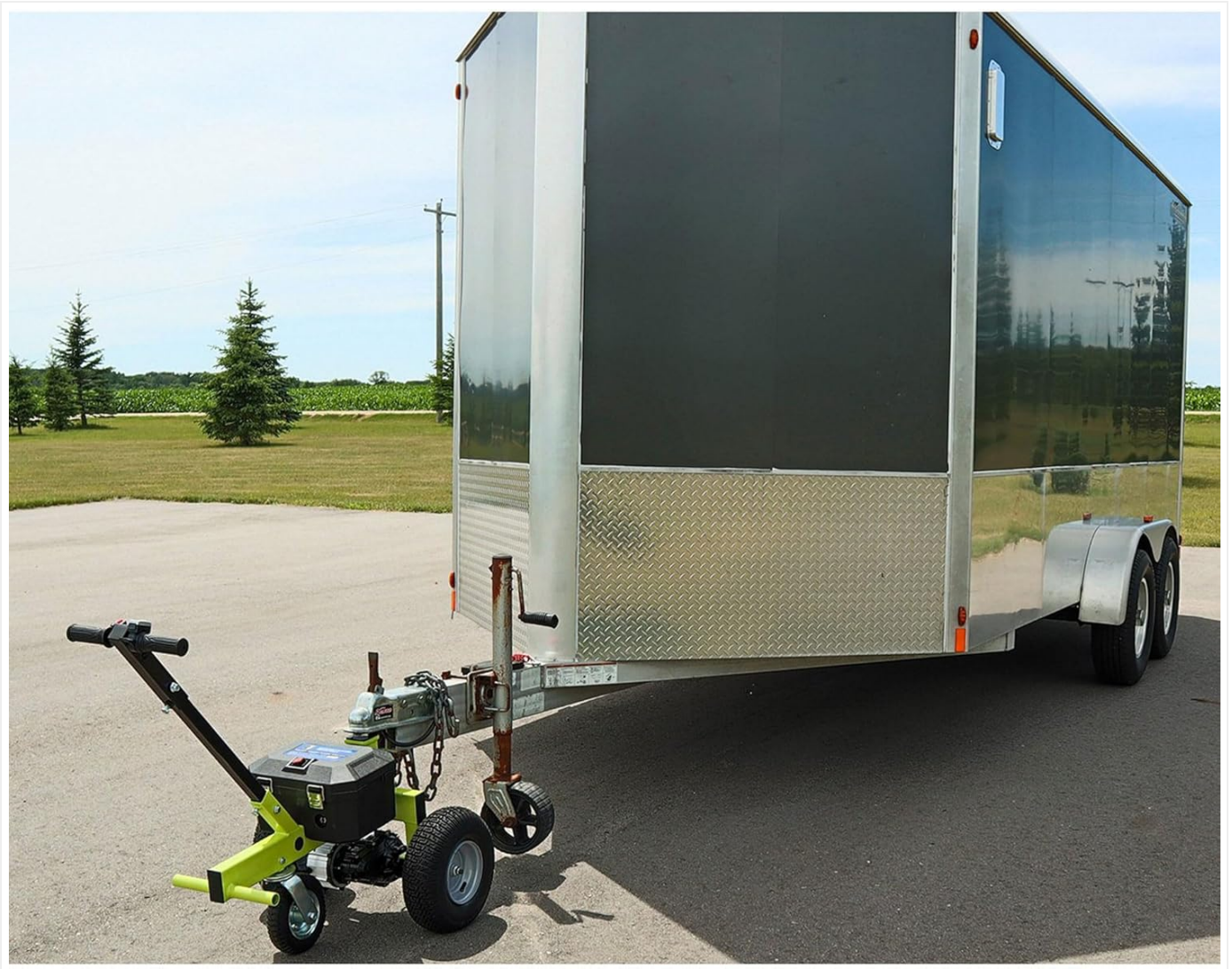
Image: The electric trailer dolly connected to a large cargo trailer, illustrating its capability to move heavy loads.
