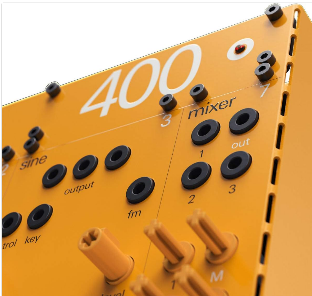
Figure 5.1: Detail of the mixer module, illustrating its inputs and output.
