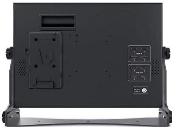
Figure 4.1: Rear view of the monitor with V-mount battery plate and power input.
